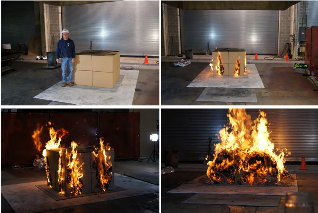
Figure 6: Heat release rate and photographs of Test 4.
