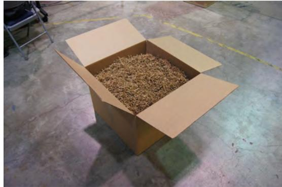
**Box #2:** Single-wall corrugated box with nominal dimensions 41 cm by 30 cm by 30 cm (16 in by 12 in by 12 in) filled with dry cotton rags. The box alone had a mass of approximately 0.8 kg (1.8 lb), and the box and rags combined had a mass of approximately 4.5 kg (10 lb). The box top was taped shut for the burns.
