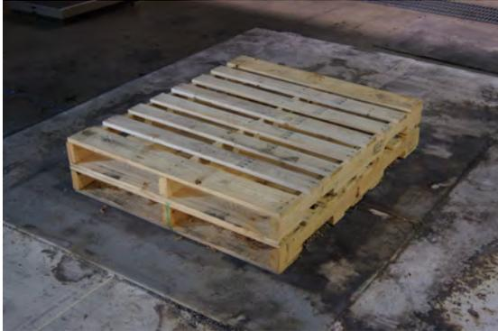
**Crib:** Pine wood crib with dimensions 56 cm by 56 cm by 46 cm (22 in by 22 in by 18 in) constructed of slats with a cross-section 3.8 cm (1.5 in) square. Its mass was approximately 39 kg (86 lb). Its moisture content was less than 5 %. It was ignited with 0.75 kg (1.7 lb) of crinkle paper stuffed in the space below the first row of slats.
