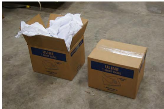
**Box #3:** Single-wall corrugated box with nominal dimensions 53 cm by 53 cm by 53 cm (21 in by 21 in by 21 in) filled with 100 rigid polystyrene cups. The corrugated box and inner liners alone had a mass of approximately 3.5 kg (7.7 lb), and the total combined mass was approximately 7.0 kg (15 lb). The top was taped shut. This item was originally developed by FM Global for use in rack storage commodity testing.
