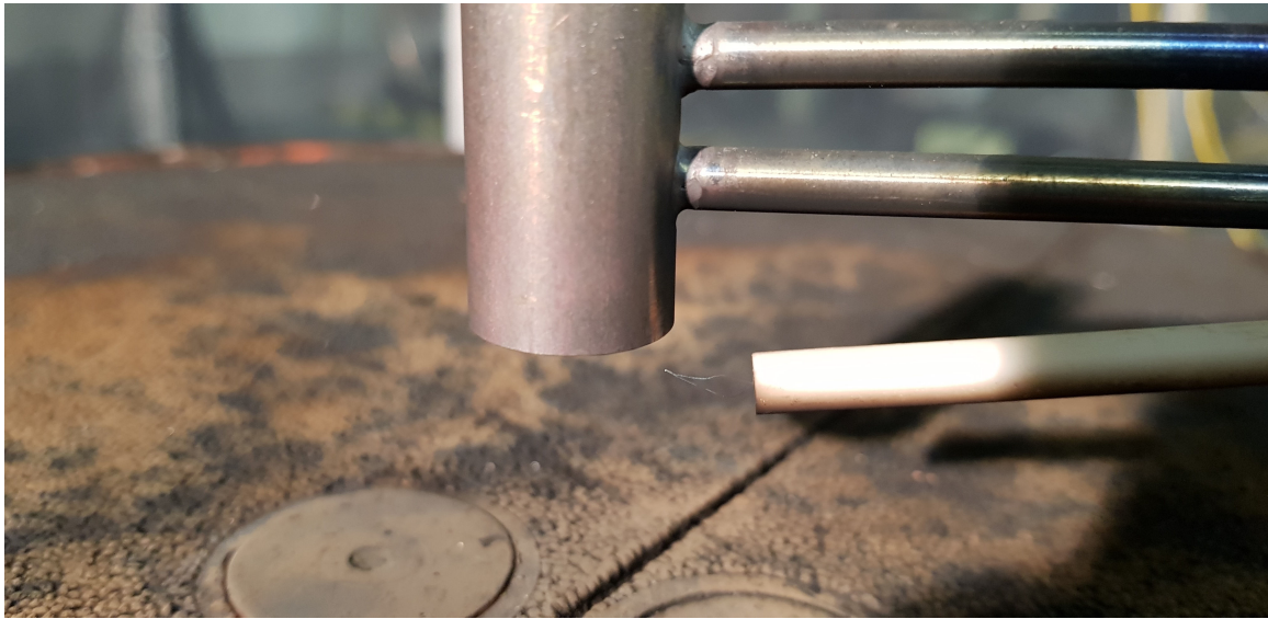
Fig. 4. Photograph of a bi-directional probe with a Type S, 25 \mu\text{m} wire diameter, bare-bead thermocouple positioned a few cm above the water-cooled, sintered-metal, 37 cm diameter, gas burner.
