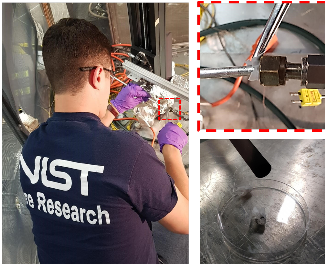
Fig. 8. Process of collecting soot from the internal walls of the quenching probe using gun cleaning patches
