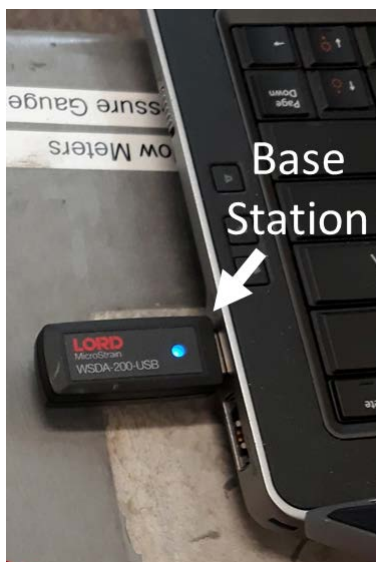
Fig. 9. The base station attached to the laptop through a USB port.
