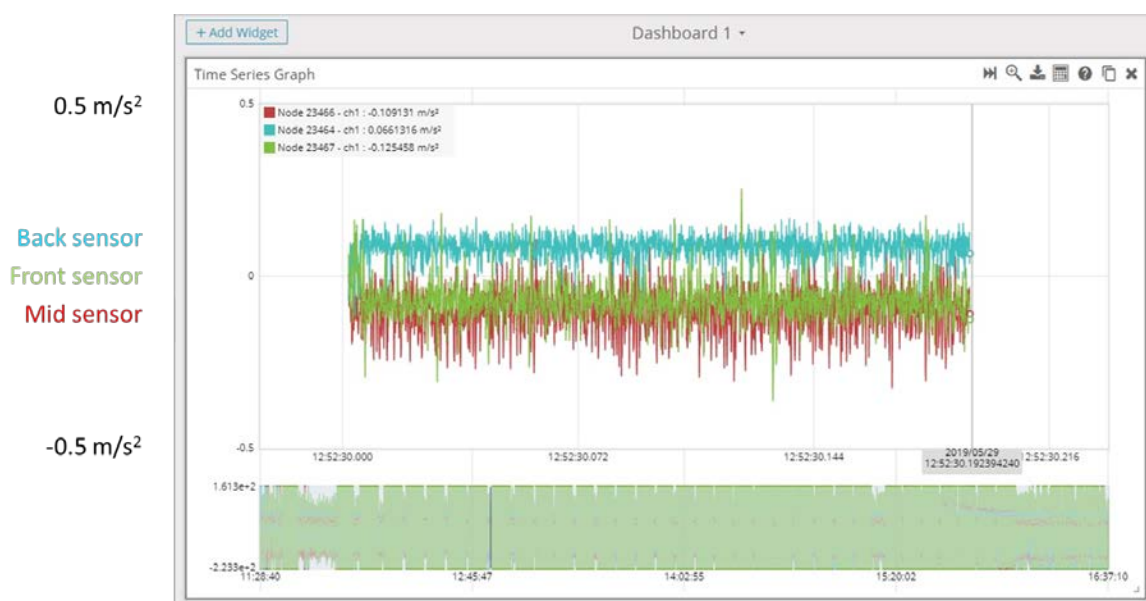
Fig. 12. Baseline data collected during a single sampling burst for 0.19 seconds for the no-flow condition in a time-series plot.
