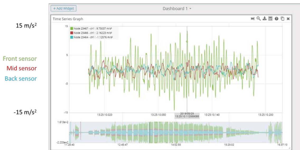
Fig. 15. Data collected (from Test 6) for a single data sampling burst for 0.19 seconds for the three accelerometers at 420 LPM (111 GPM) in a time-series plot from which the standard deviation of the signal was determined.
