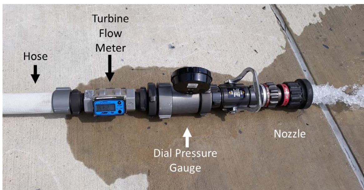
Fig. 10. Nozzle, dial pressure gauge, and turbine reference flow meter at the front, or downstream, end of the fire hose.
