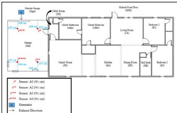
**Figure 99a.** Generator, exhaust direction, and sensor array layout during Case 45 Test 2 – G7b UL 2201.
