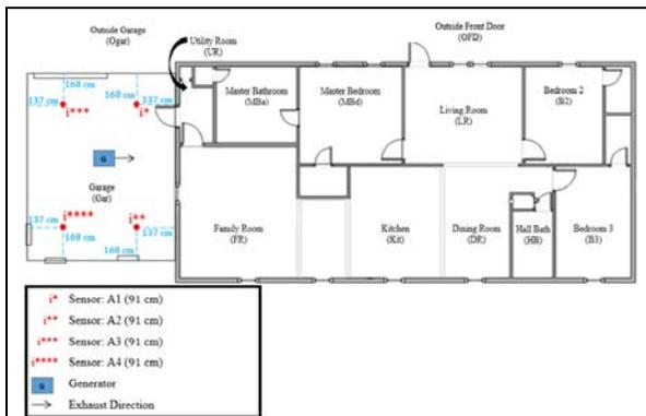
**Figure 78a.** Generator, exhaust direction, and sensor array layout during Case 32 Test 1 – G6 G300.
