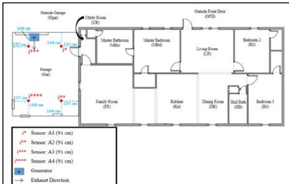
**Figure 88a.** Generator, exhaust direction, and sensor array layout during Case 37 Test 1 – G15 G300.
