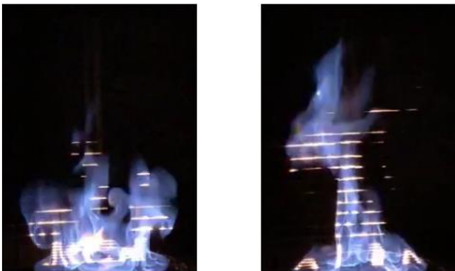
Figure 4. Two images of the glowing filaments mounted above the central plane of the methanol pool fire.
