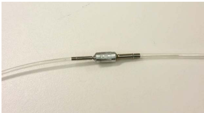
Figure 6.8 Restrictor built for experiments.
