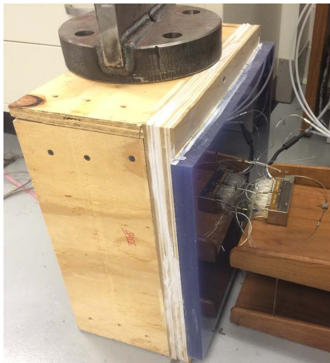
Figure 4.1. An experimental device for fluctuating pressure generation.
