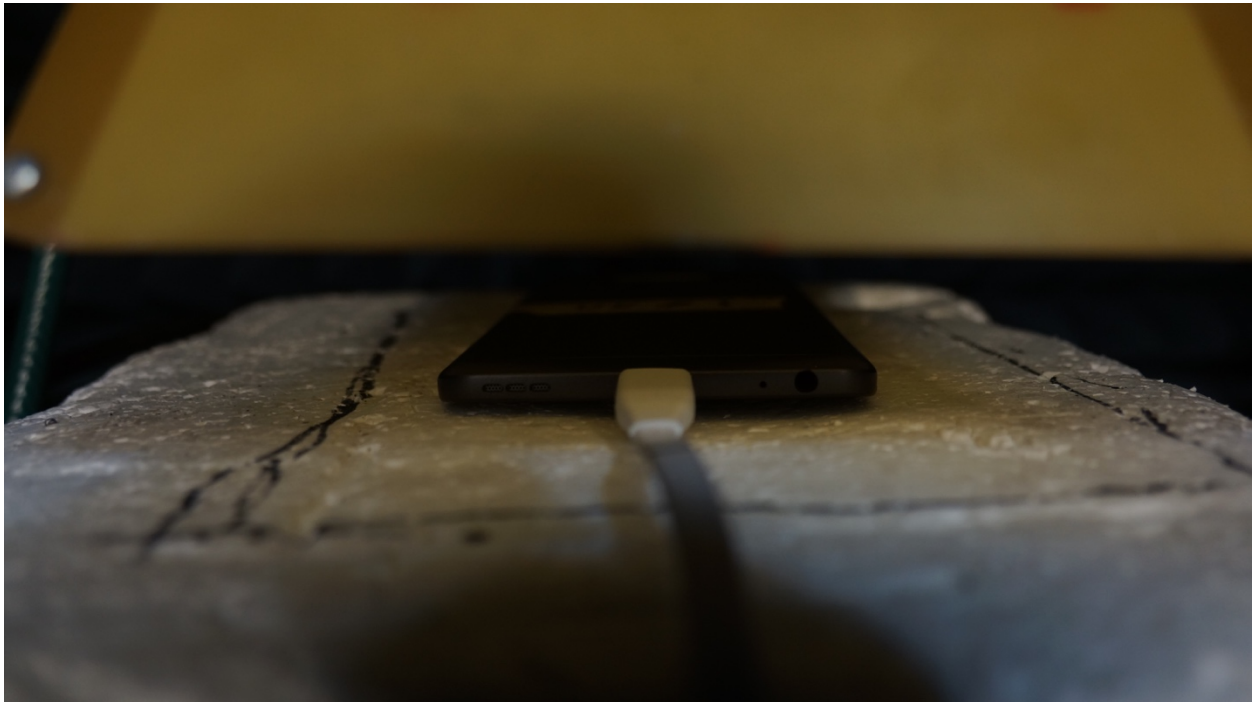
Figure 10. A UE positioned approximately 3 cm underneath the horn antenna during emission measurements.
