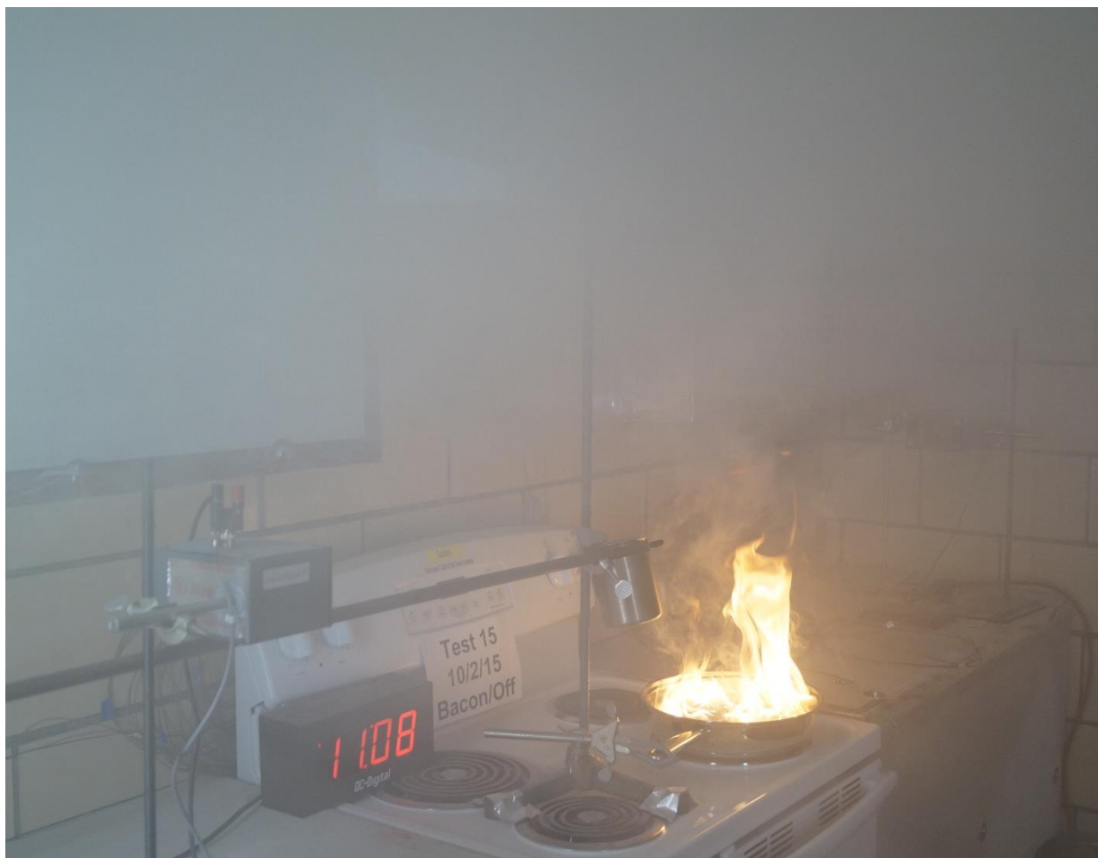
Figure 30 A photograph of ignited bacon during Test 15 showing the visual obscuration of the laboratory due to accumulated smoke.
