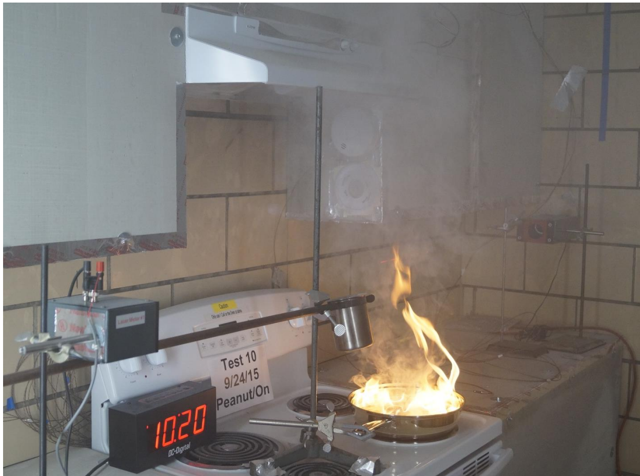
Figure 7 Ignited peanut oil during Test 10 before extinguishment.
