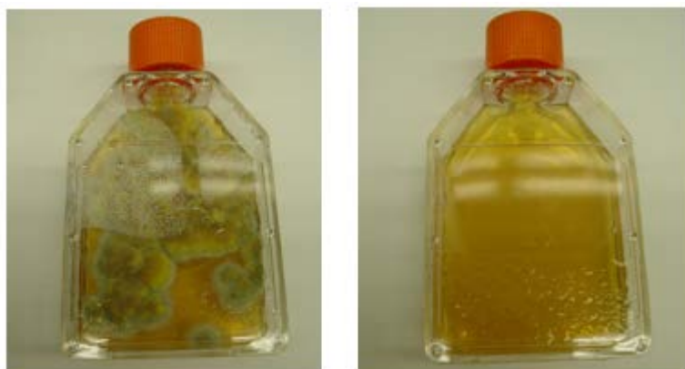
Figure 5: Accelerated microbial growth environments analyzing a (left) normal SRM sample and (right) a sterilized SRM sample.
