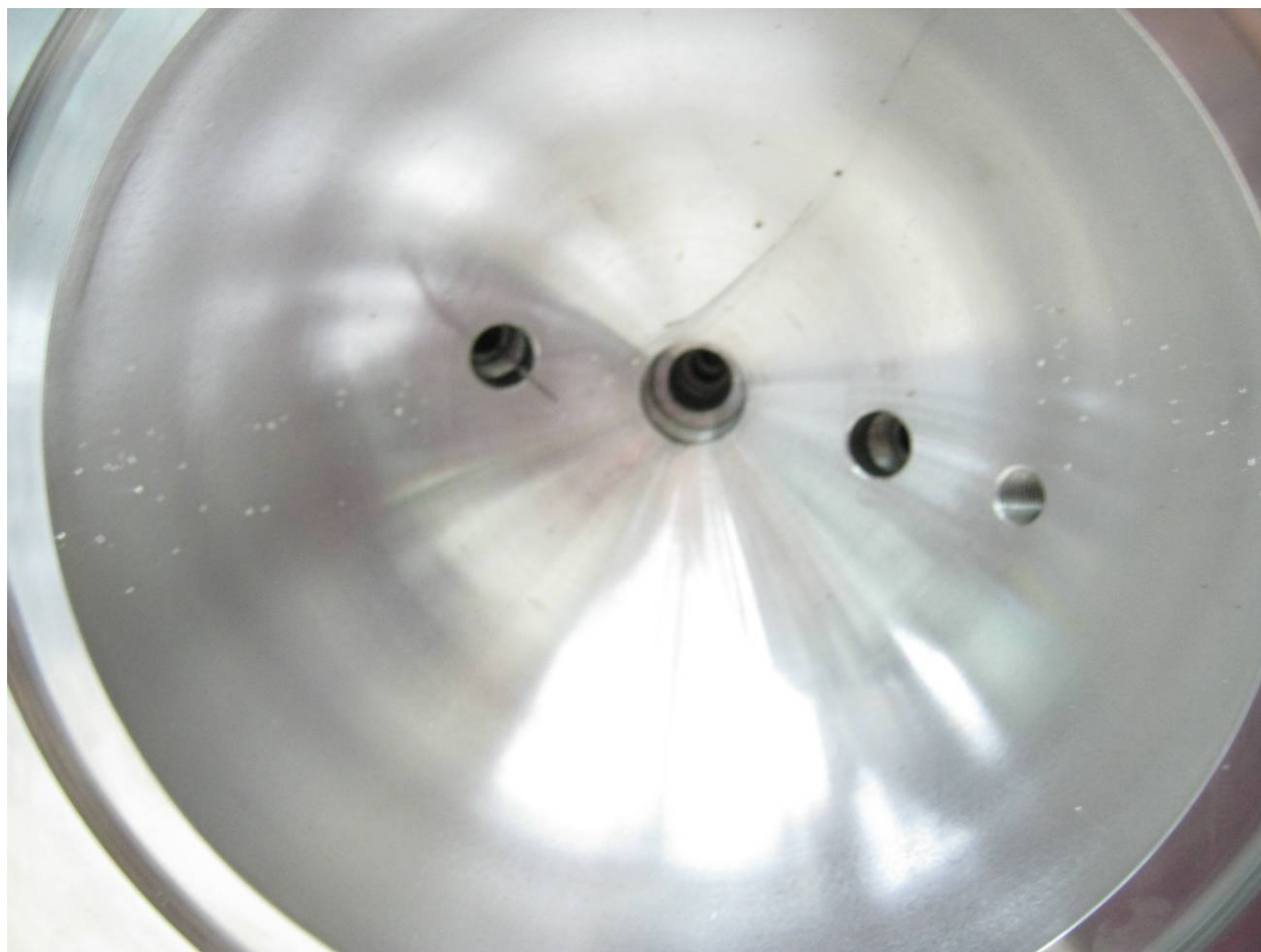
Figure 8 - Top, inside surface of 2-L chamber after several tests with the platinum igniter.
