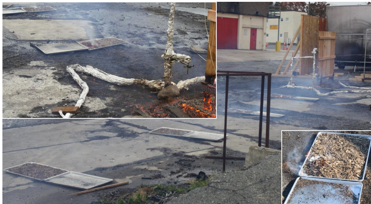
Figure 15 Photographs from Test 9 (cedar at 0°, 13.5 m/s) showing three perspectives on the first (3.05 m) target pan with burning mulch and airborne firebrands.
