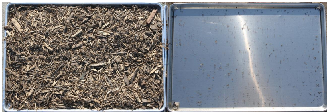
Figure 4 Photographs of a pair of firebrand targets after Test 7 (cedar at 45°, 13.5 m/s). One pan is filled with about 2 cm of mulch (left) and the other contains about 4 mm of water (right). These were placed in 3.05 m intervals downwind of the trailing edge of the fence.
