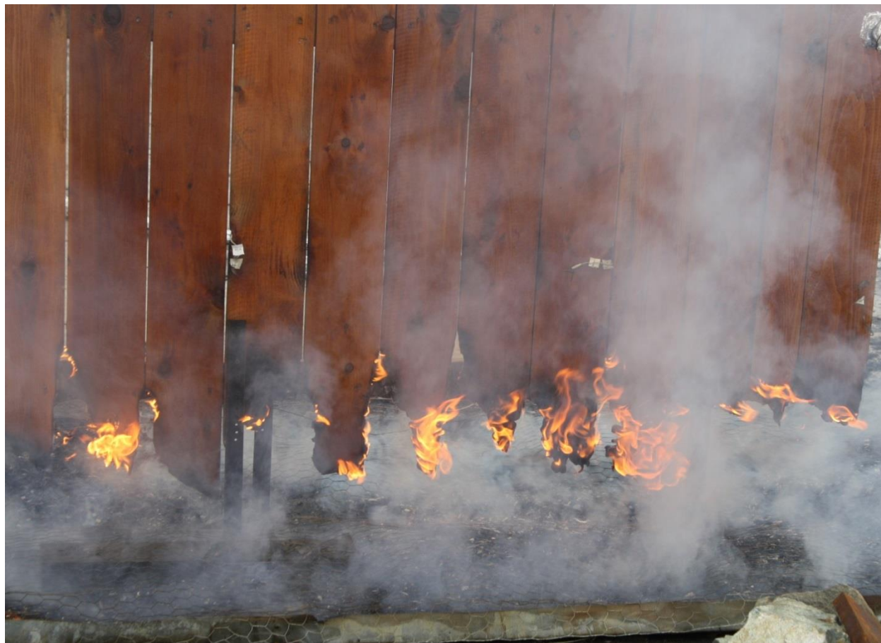
Figure 13 Photograph from Test 13 (preservative-coated cedar at 0^\circ , 13.5 m/s) showing flames attached to several fence boards and a significant amount of material burned away from the board ends. Wind direction was left to right.
