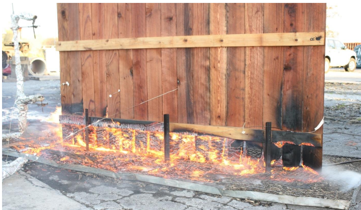
Figure 14 Photograph from Test 12 (preservative-coated redwood at 0°, 13.5 m/s) showing substantial burning of the lower 2/3 of the structure side of the fence after the fire progressed (from right to left) to the end.
