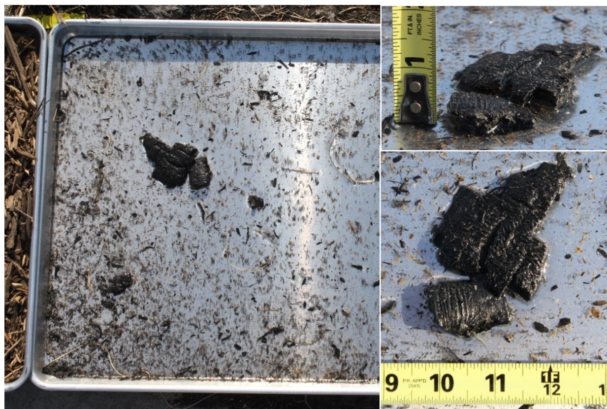
Figure 16 A photograph of a fence-generated firebrand in the first (3.05 m from fence) water pan surrounded by smaller mulch-generated firebrands produced during Test 12 (preservative-coated redwood at 0°, 13.5 m/s). Additional photographs provide size reference for the firebrand.
