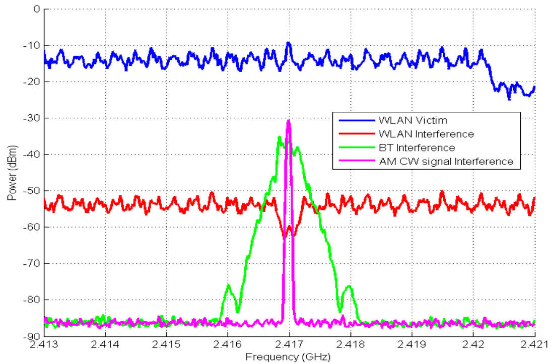
Figure 5. 8 MHz of the spectrum centered on the carrier frequency of the Bluetooth® and AM interference signals.
