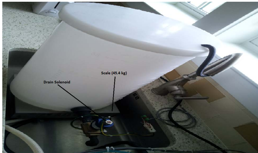
Figure 16. Kitchen sink water measurement apparatus
