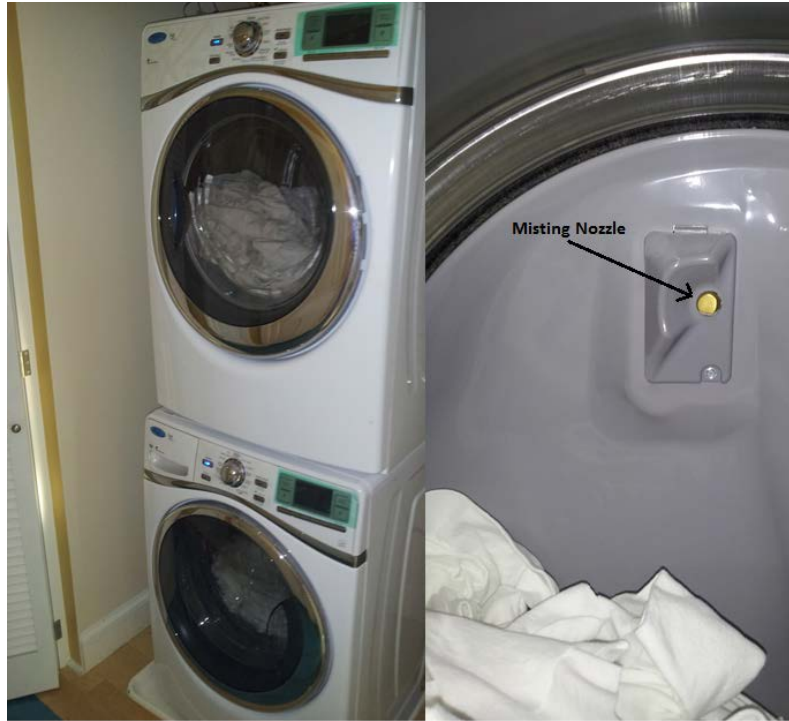
Figure 21. The dryer, modified misting nozzle, and the washer
