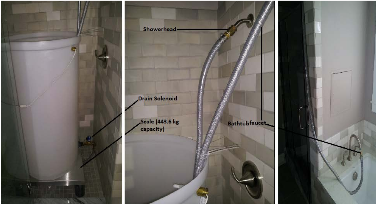
Figure 15. Master bathroom water measurement apparatus
