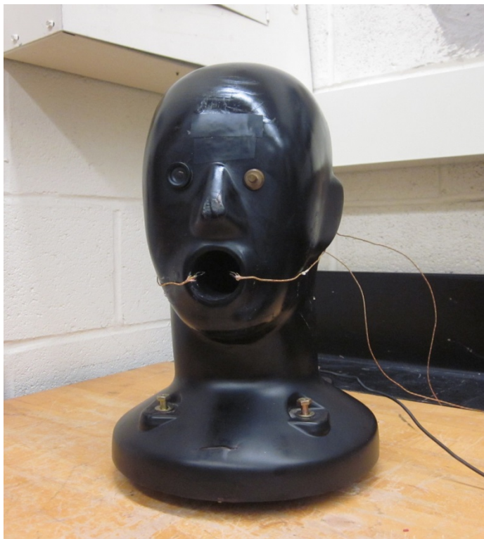
Figure 3 Mannequin headform with thermocouples inside mouth.
