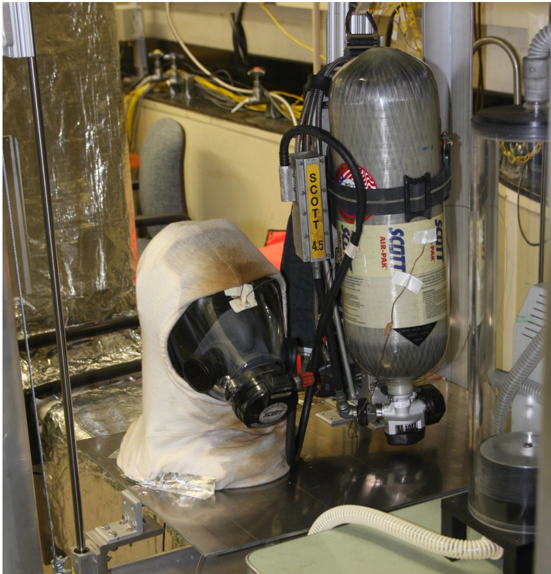
Figure 2 SCBA equipment on the flow loop testing platform
