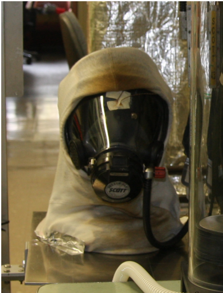
Figure 4 Thermocouples placed on SCBA facepiece
