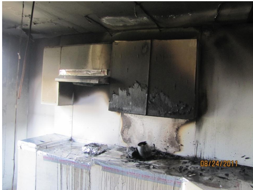
Figure 56. Post-fire photo of experiment B1_1 (Laminated pressboard, scenario 1).
