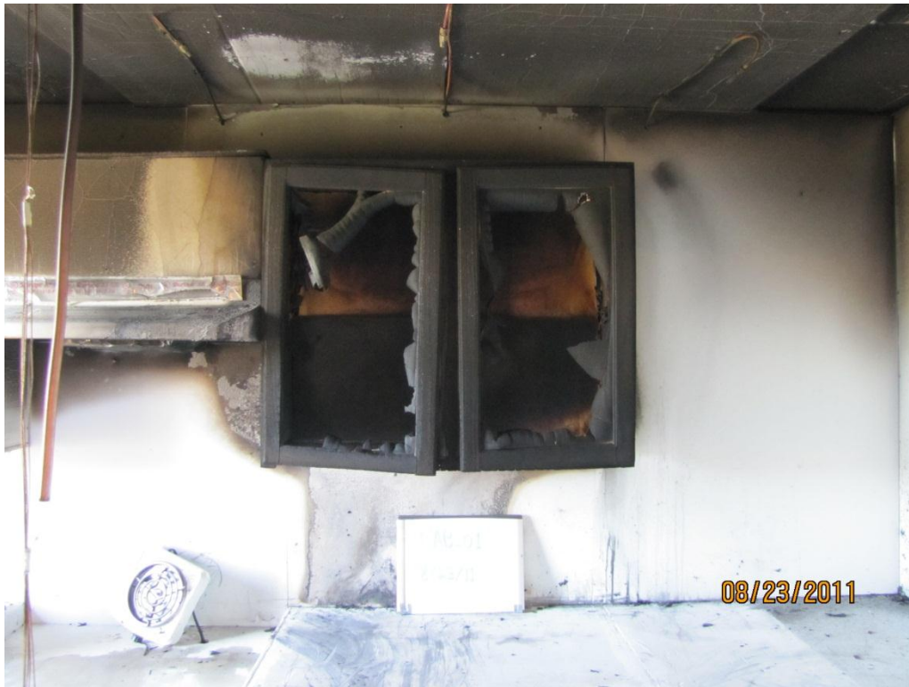
Figure 45. Post-fire photo of experiment A1_1 (Oak/pressboard, scenario 1).
