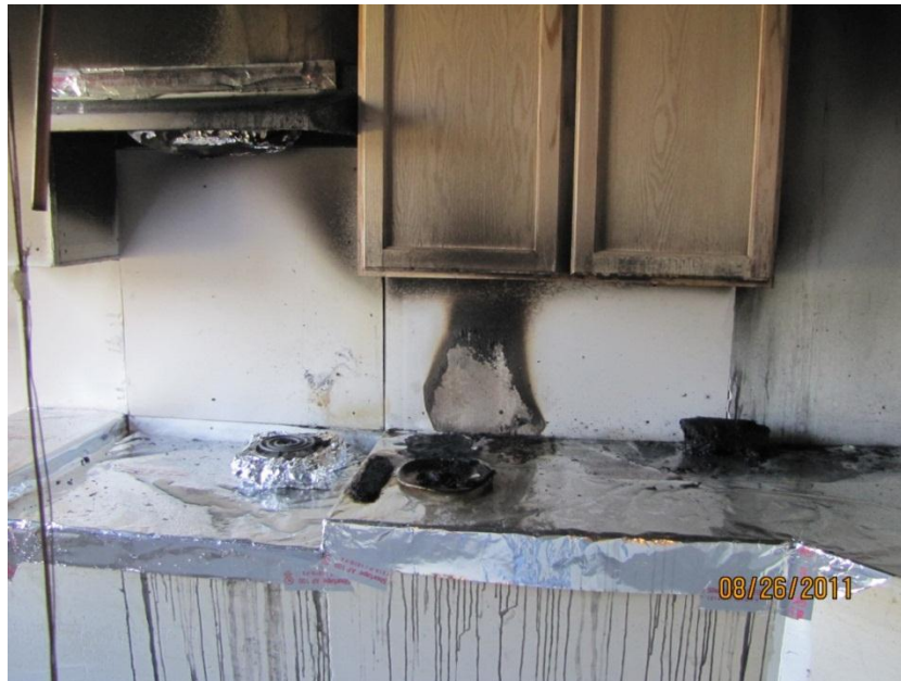
Figure 50. Post-fire photo of experiment A2_1 (Oak/pressboard, scenario 2).
