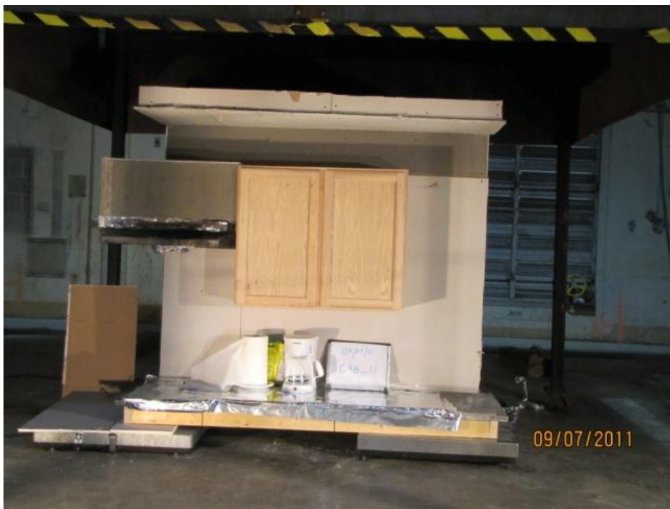
Figure 9. Kitchen counter and cabinet mockup. The counter level rests on load cells, and the entire mockup fits under the furniture calorimeter hood.
