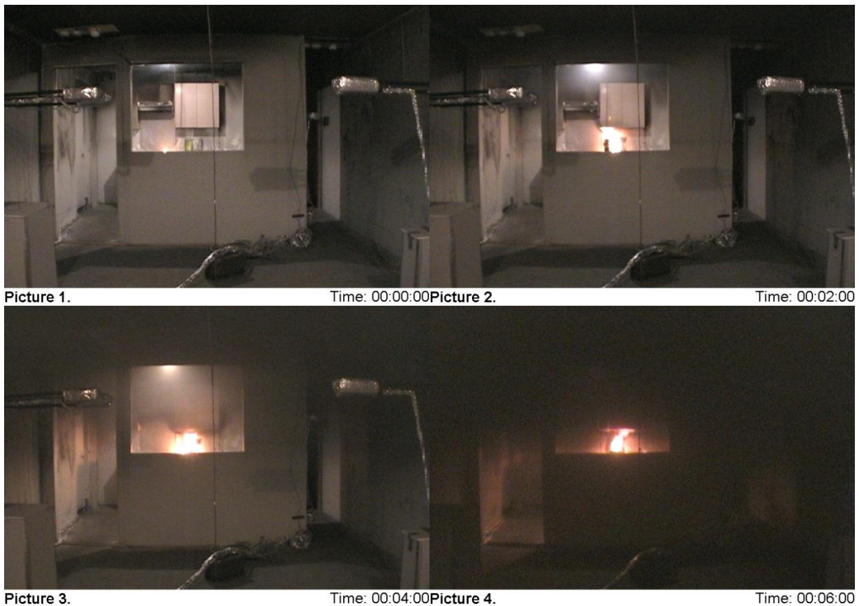
Figure 55. Photo sequence for experiment B1_1 (Laminated pressboard, scenario 1).
