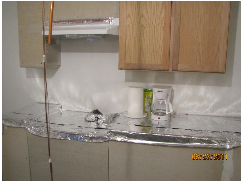
Figure 22. Configuration of kitchen counter and cabinet with ignition scenario 1 shown.
