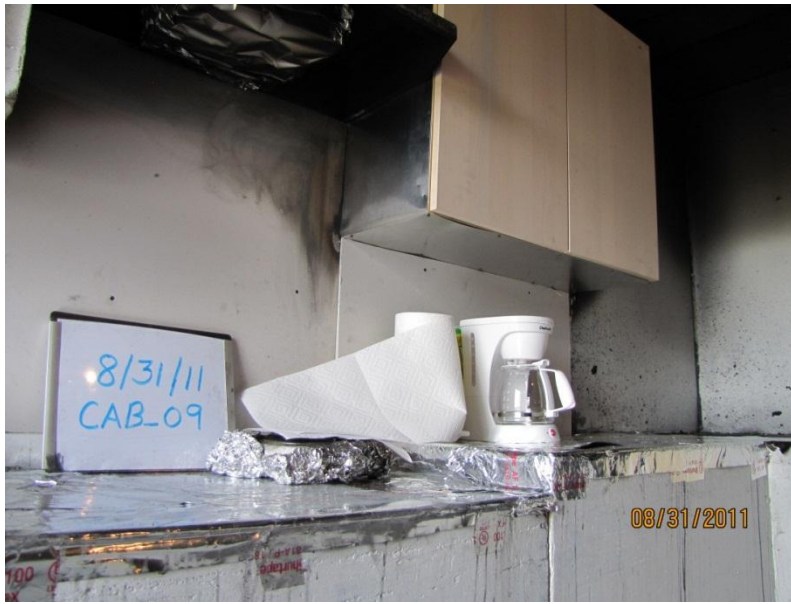
Figure 70. Pre-fire photo of experiment B3_1 (Oak/pressboard with sheet metal barrier, scenario 1).
