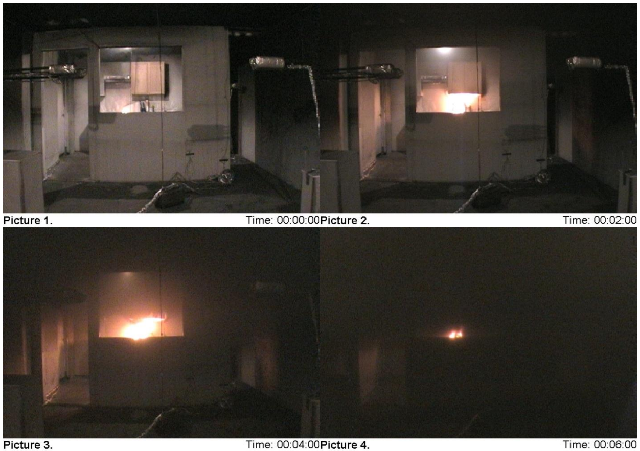
Figure 52. Photo sequence for experiment A2_2 (Oak/pressboard, scenario 2).
