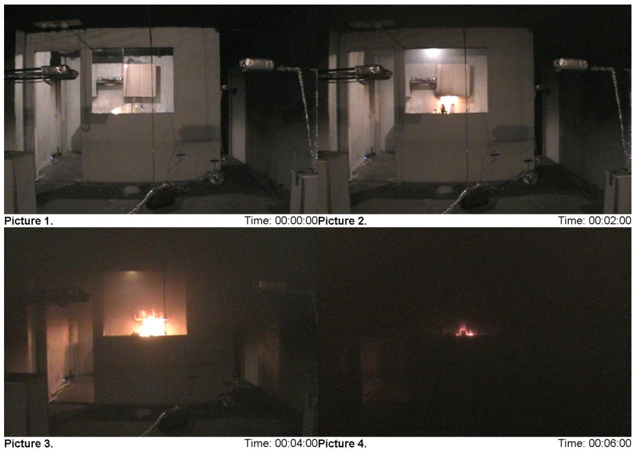
Figure 58. Photo sequence for experiment B1_2 (Laminated pressboard, scenario 1).
