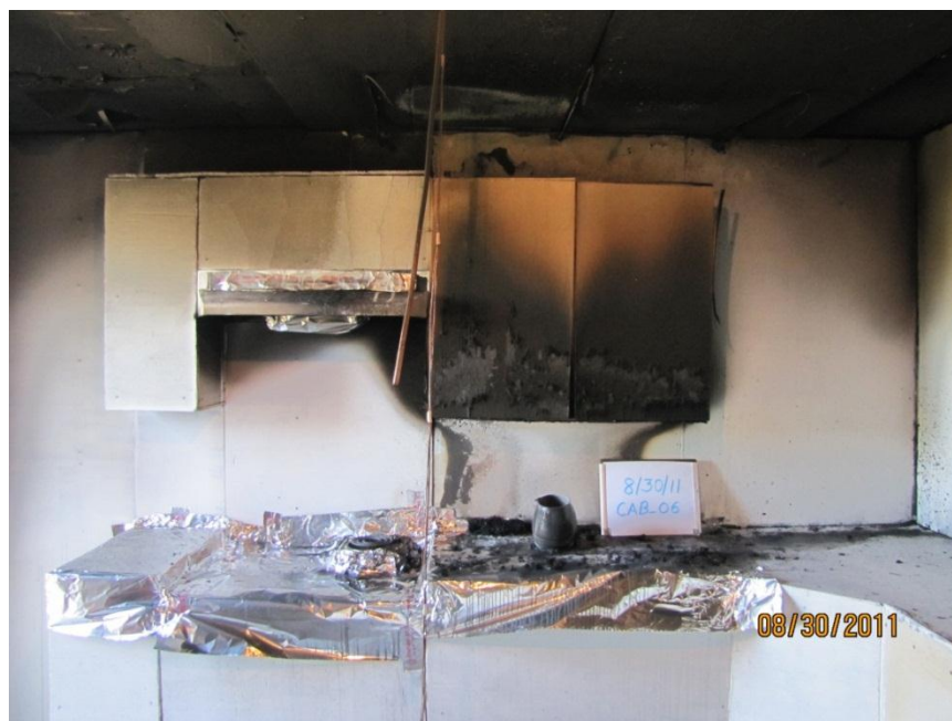
Figure 59. Post-fire photo of experiment B1_2 (Laminated pressboard, scenario 1).
