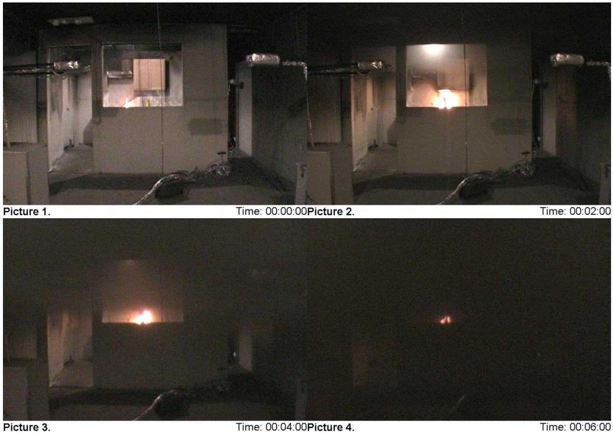
Figure 49. Photo sequence for experiment A2_1 (Oak/pressboard, scenario 2).
