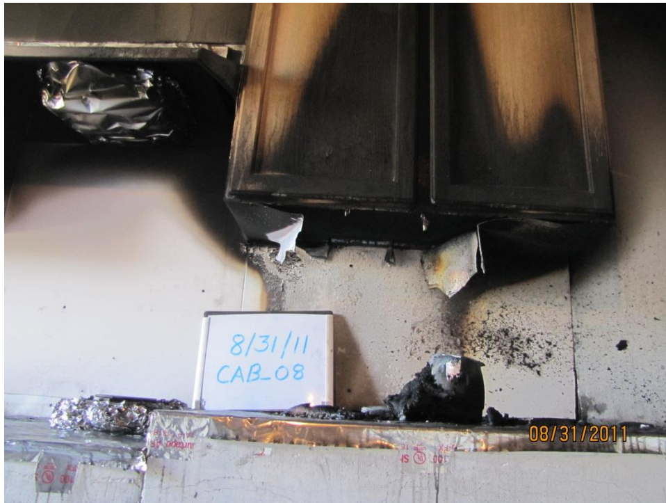
Figure 67. Post-fire photo of experiment A3_1 (Oak/pressboard with sheet metal barrier, scenario 1).
