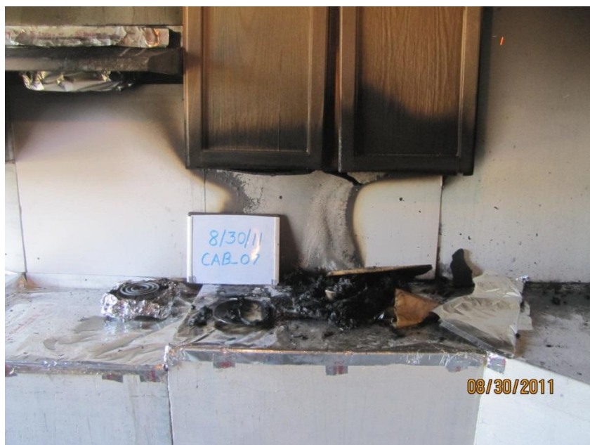
Figure 53. Post-fire photo of experiment A2_2 (Oak/pressboard, scenario 2).
