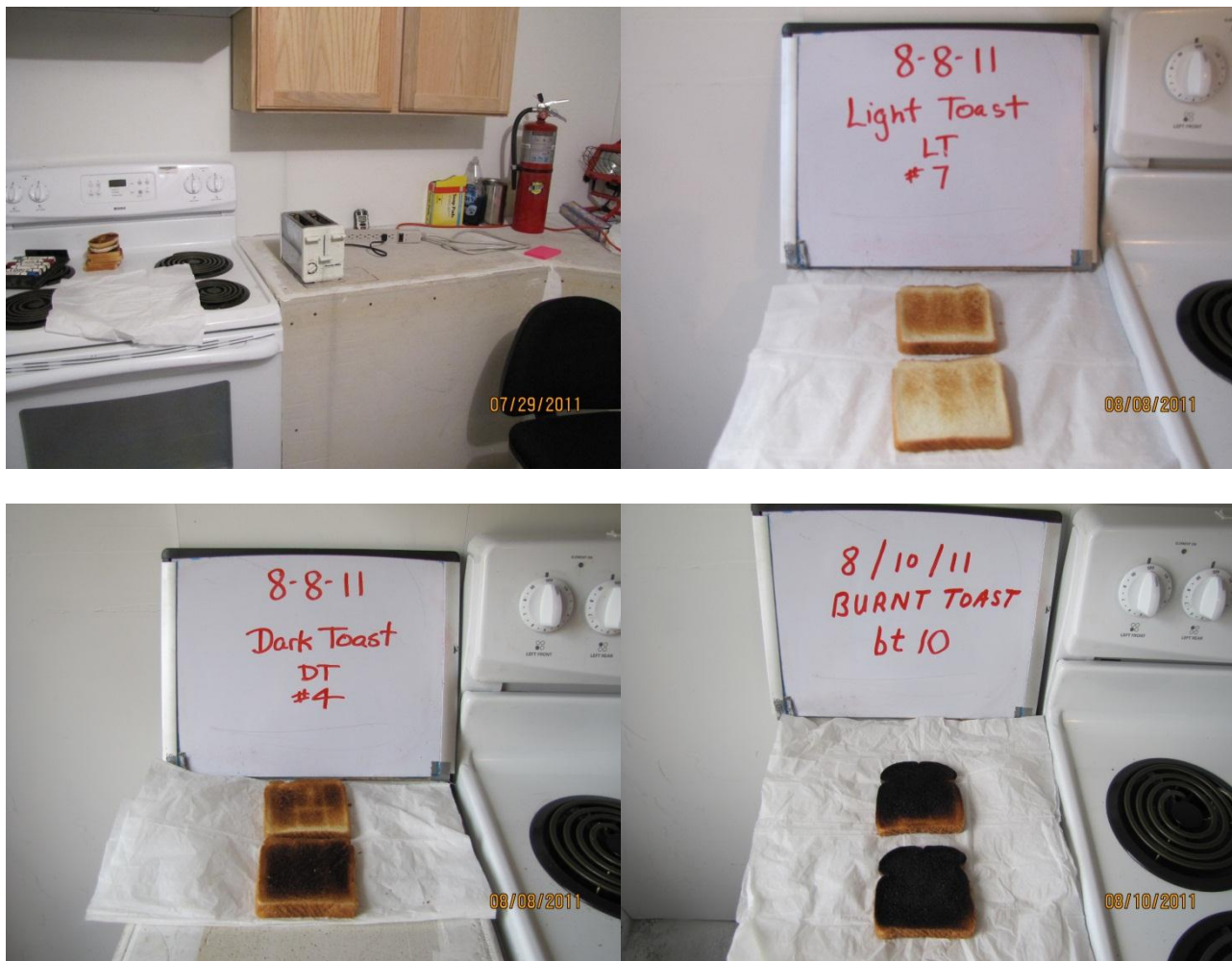
Figure 14. Toasting bread configuration and toasted bread exemplars. Toasting bagel
