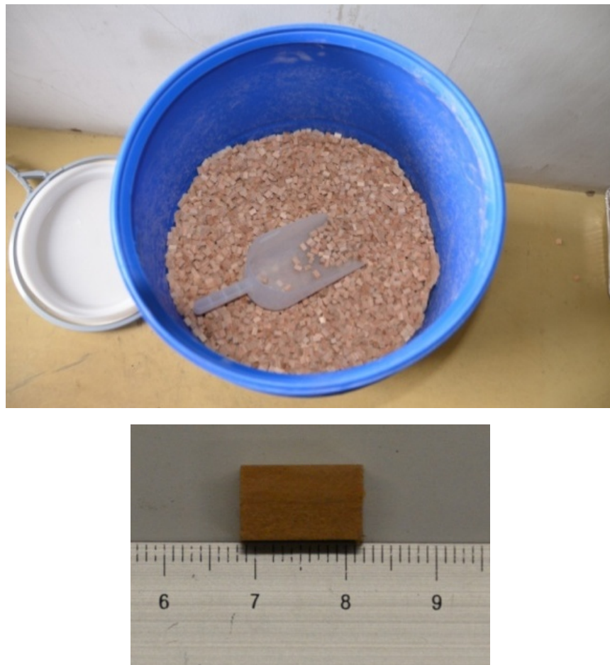
Figure 4 Picture of wood pieces (bulk – image on top shows pieces inside 215 L drum; 571 mm diameter opening) needed to feed the full-scale Continuous Feed Firebrand Generator. Detailed image (bottom) of a single wood piece along with a metric ruler in cm.
