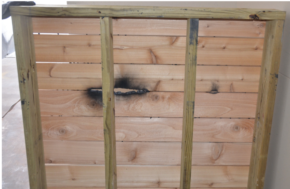
Figure 15 Picture of the underside of the decking assembly (cedar); overall view.
