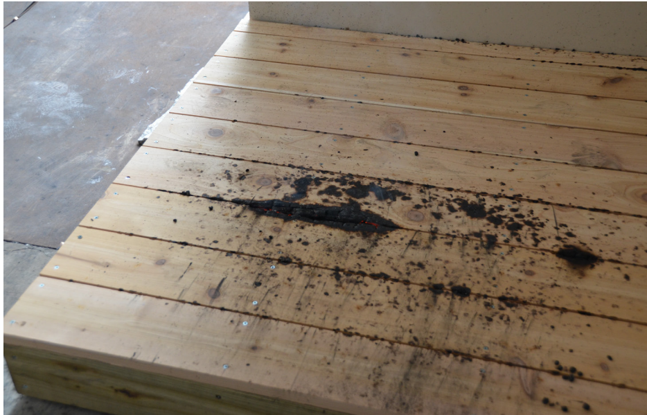
Figure 11 Cedar decking assembly after accumulated firebrands were swept off and wind tunnel was off. Smoldering ignition is still occurring.
