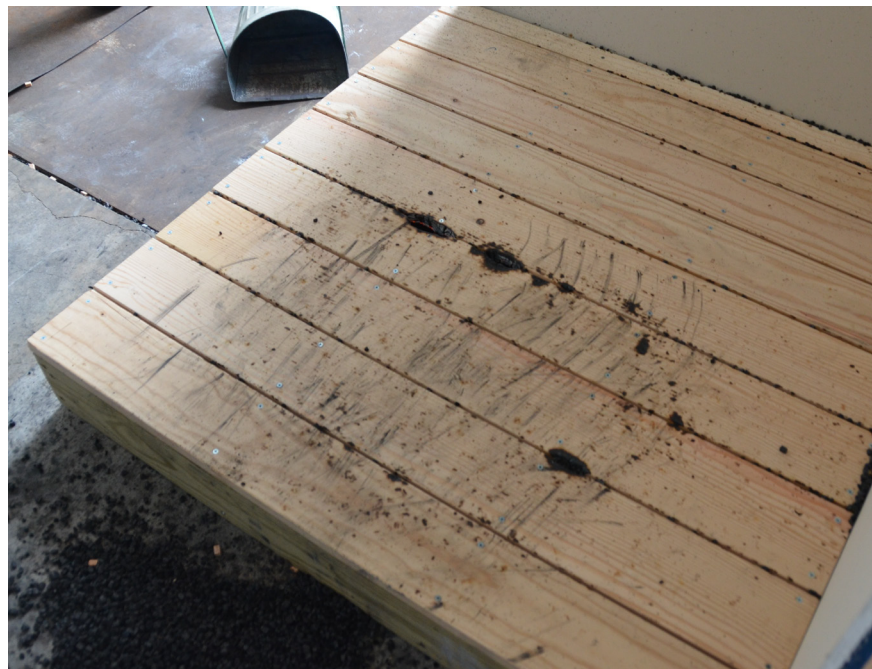
Figure 12 Douglas-Fir decking assembly after accumulated firebrands were swept off and wind tunnel was off. Smoldering ignition is still occurring.
