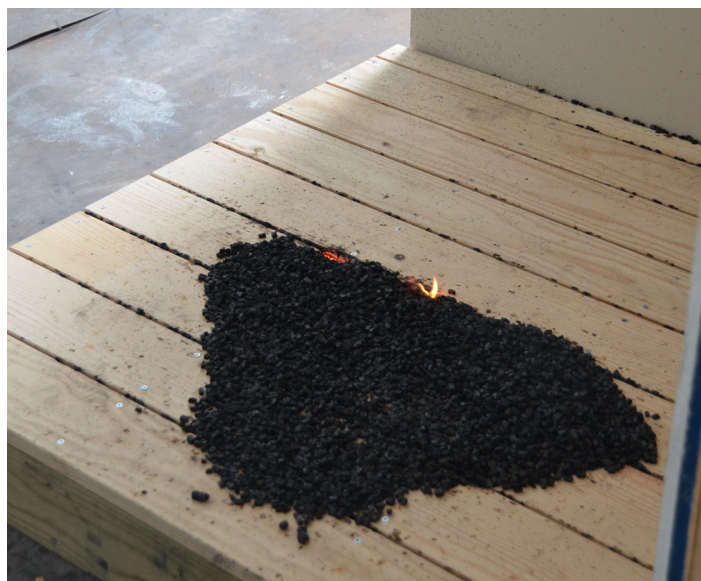
Figure 9 Flaming ignition of Douglas-Fir decking assembly.
