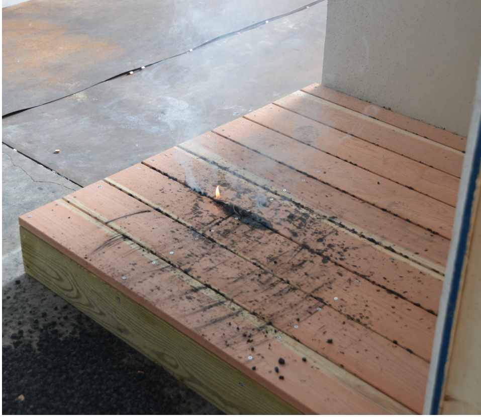
Figure 13 Redwood decking assembly after accumulated firebrands were swept off and wind tunnel was off. Smoldering ignition and local flaming ignition is still occurring.
