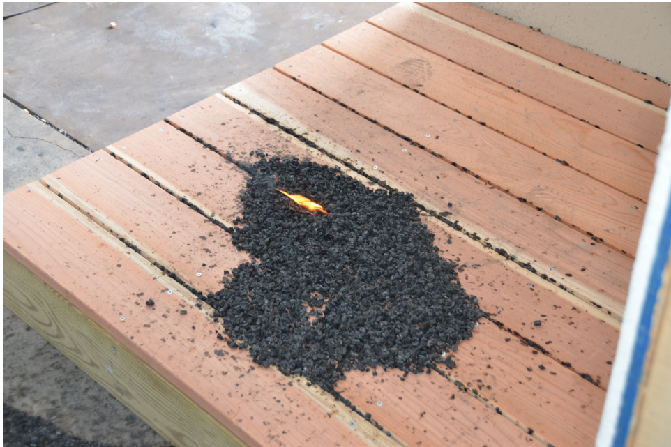
Figure 10 Flaming ignition of Redwood decking assembly.
