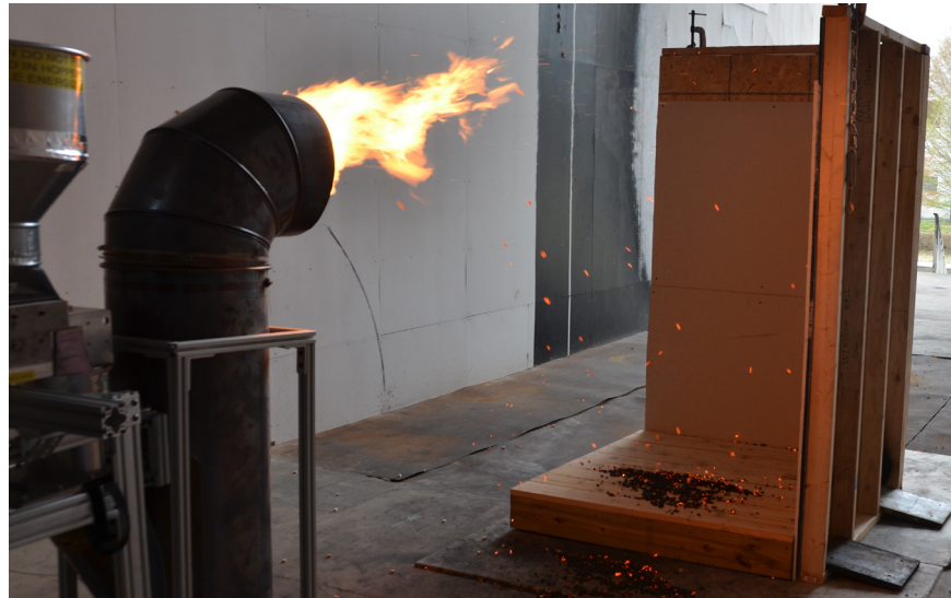
Figure 7 Picture of a typical experiment exposing a decking assembly to continuous wind-driven firebrand showers. In this particular experiment, cedar was used as the decking material.
