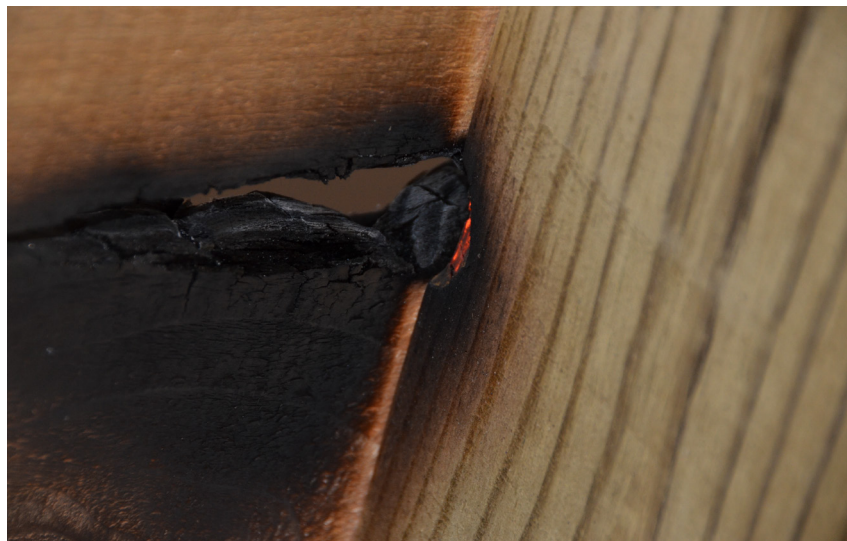
Figure 16 Detail of the underside of the decking assembly (cedar). The ignition process was observed to spread to the wood supporting members.
