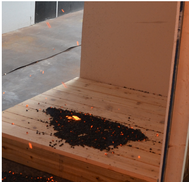
Figure 8 Flaming ignition of Cedar decking assembly.
