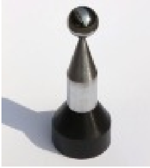
(a) Case study 1 – CMM calibration master ball
