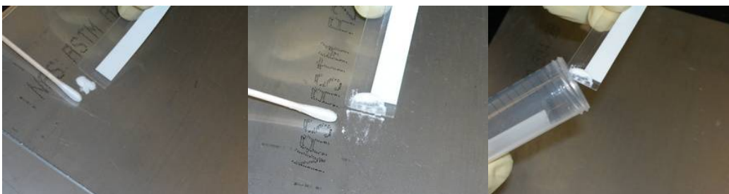
Figure 1- Demonstration of ASTM E2458-10 Method A for sampling visible powders from nonporous surfaces using a sterile non-cotton swab and laminated card
