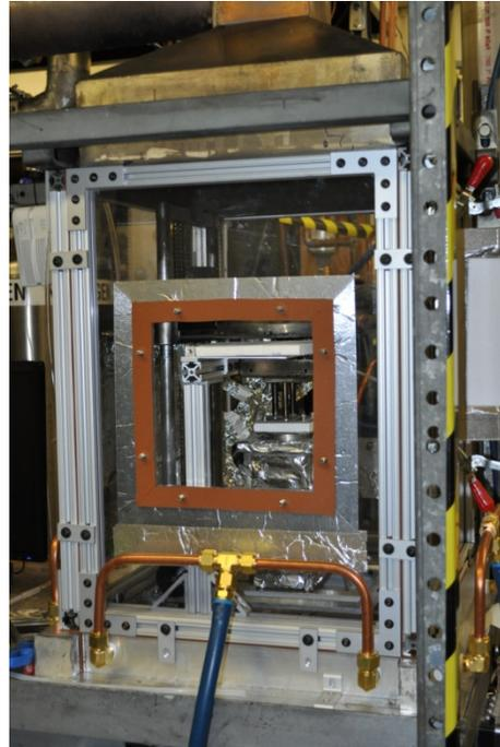
**Figure 1. Modified Cone Calorimeter**
