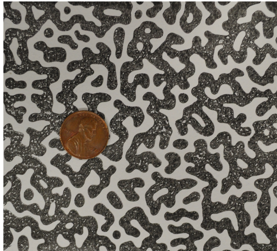
Figure 4: Pattern used for digital image correlation measurements as painted on a gusset plate specimen. A 19.0 mm diameter coin is shown for reference.
