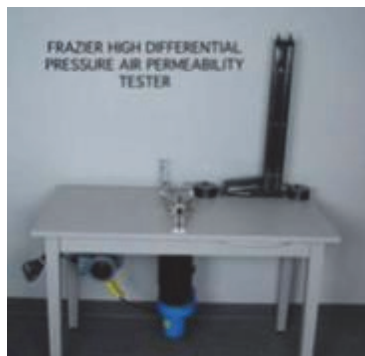
Figure 16. Photograph of the electronic high differential pressure instrument for measuring air permeability.
