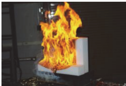
Figure 60. A test with formulation C1 few seconds before extinguishing the sample. At this stage flaming liquid material is dripping to the underlying tray but there is no pool fire with sustained flaming that can boost the heat release rate through a feed-back effect.
