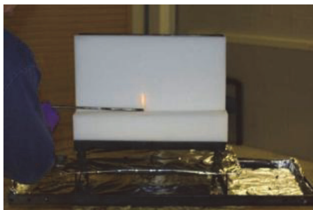
Figure 12. Photo of test with formulation C1 a few seconds before extinguishing the sample. At this stage, flaming liquid material is dripping to the underlying tray, but there is no pool fire (which would sustain flaming and boost the heat release rate through a feedback effect).
