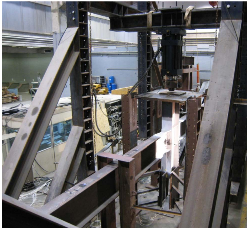
Figure 3–5 Photograph of the RBS specimen
