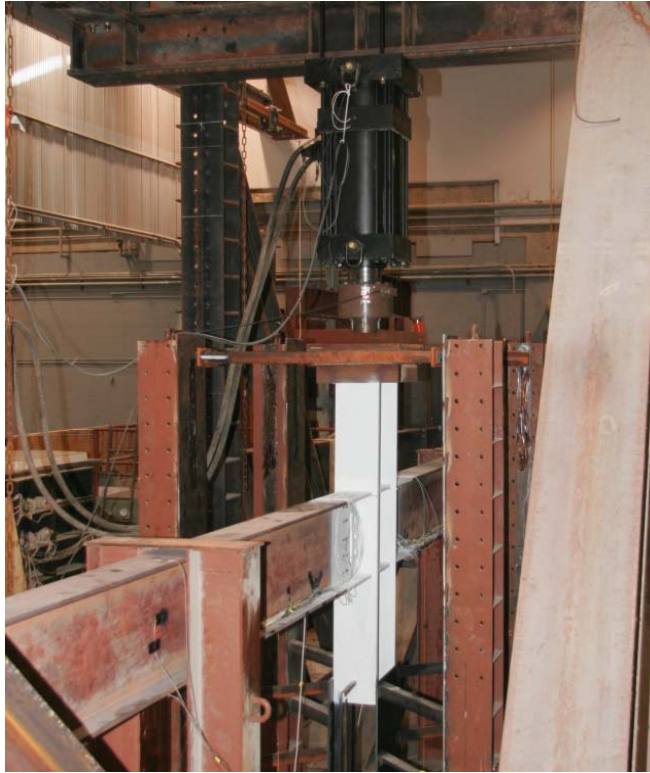
Figure 3–4 Photograph of the WUF-B specimen
