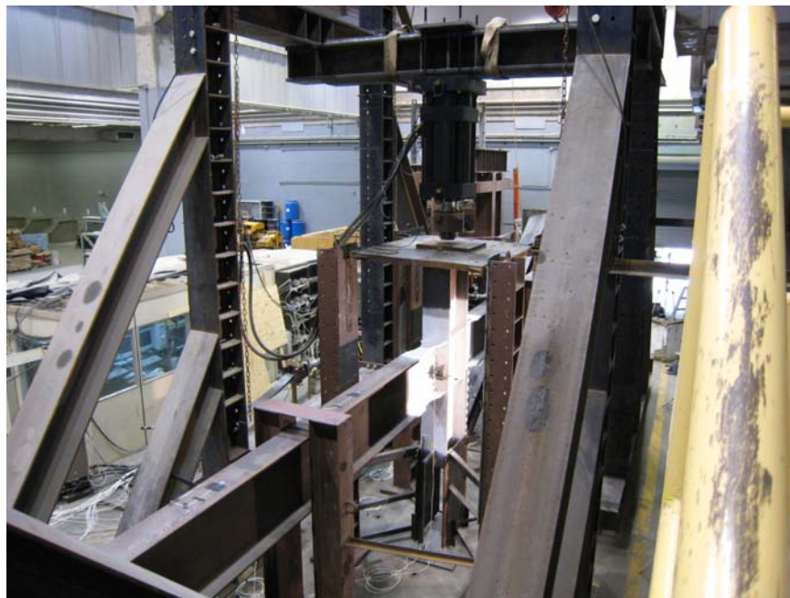
Figure 4–16 Overall view of the RBS test specimen
