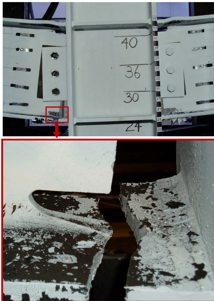
Figure 4–2 Failure mode of the WUF-B specimen
