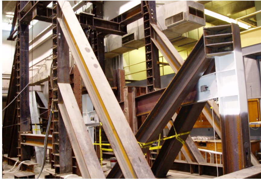
Figure 4–1 Overall view of the WUF-B specimen subjected to large displacements
