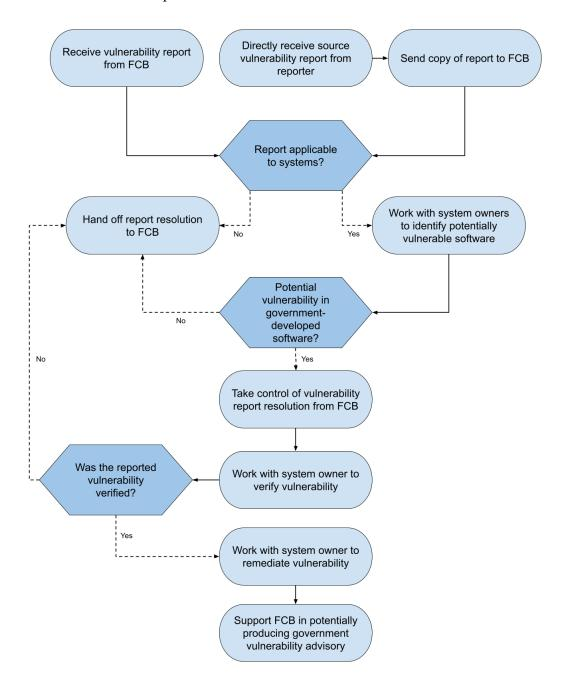
Fig. 4. Process flow specification for VDPO operational duties
