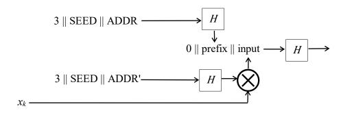
Figure 5: XMSS hash computation with prefix and bitmask
