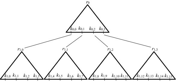
Figure 4: A two-Level Merkle tree
