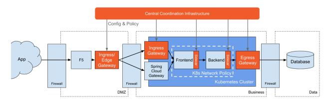
Fig. 5. Policy deployment for a three-tier application
