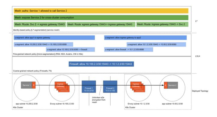
Fig. 3. Multi-tier policies for a hybrid application environment
