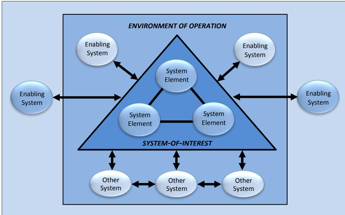
FIGURE 2: SYSTEMS ENGINEERING VIEW OF THE SYSTEM-OF-INTEREST
