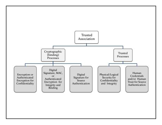
Figure 1: The Trusted Association and Supporting Processes
