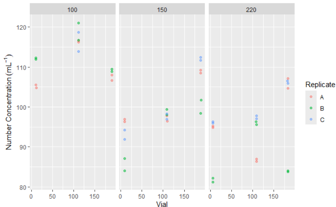
Figure 13. Particle number concentration data for the nominally 100 \mu\text{m} , 150 \mu\text{m} , and 220 \mu\text{m} sized particles. The vial index is on the x-axis, number concentration is on the y-axis, and replicate is indicated by color.
