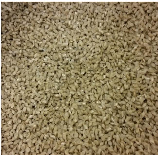
Fig. 5. Chopped and bagged pellets of PVC SRM 2861.
