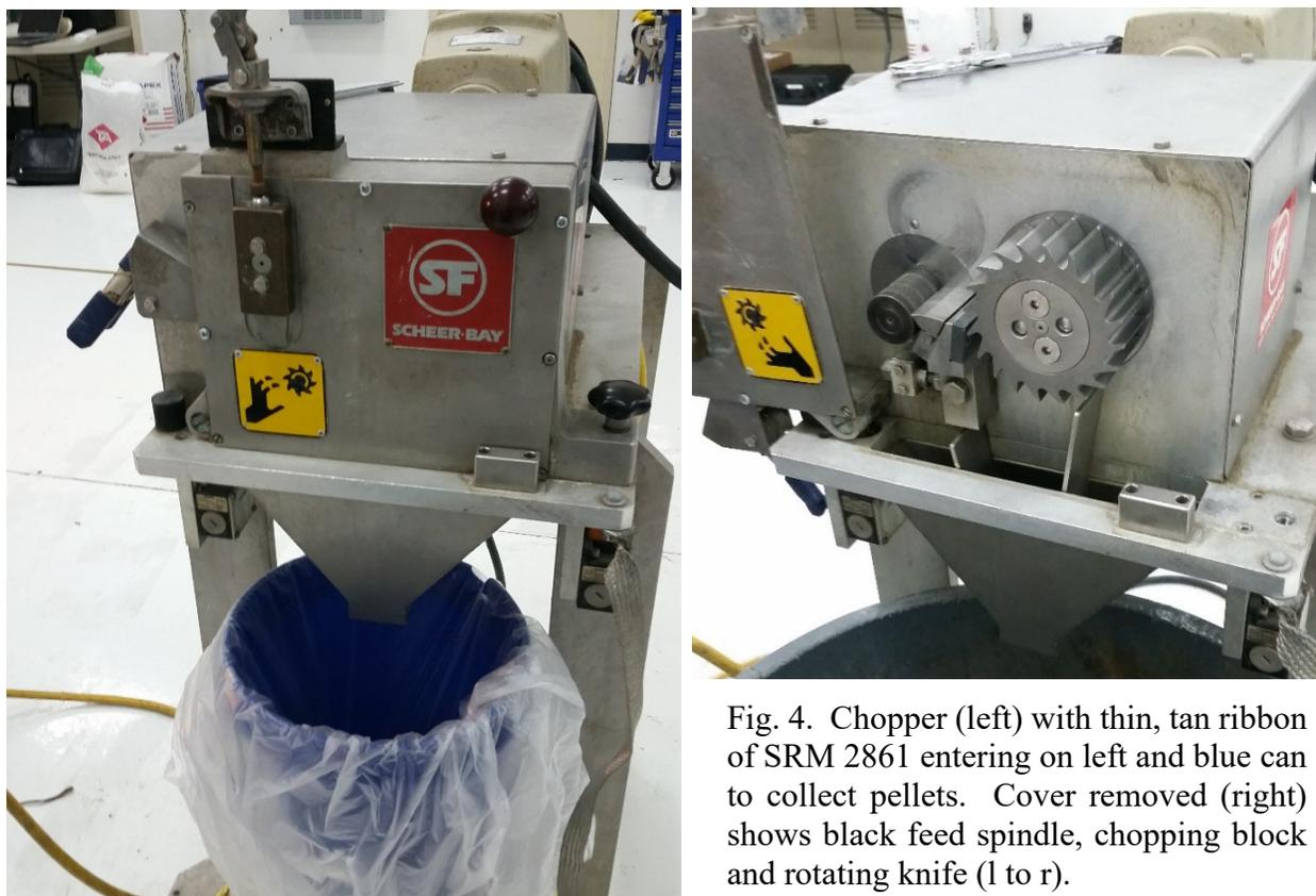
Fig. 4. Chopper (left) with thin, tan ribbon of SRM 2861 entering on left and blue can to collect pellets. Cover removed (right) shows black feed spindle, chopping block and rotating knife (l to r).
