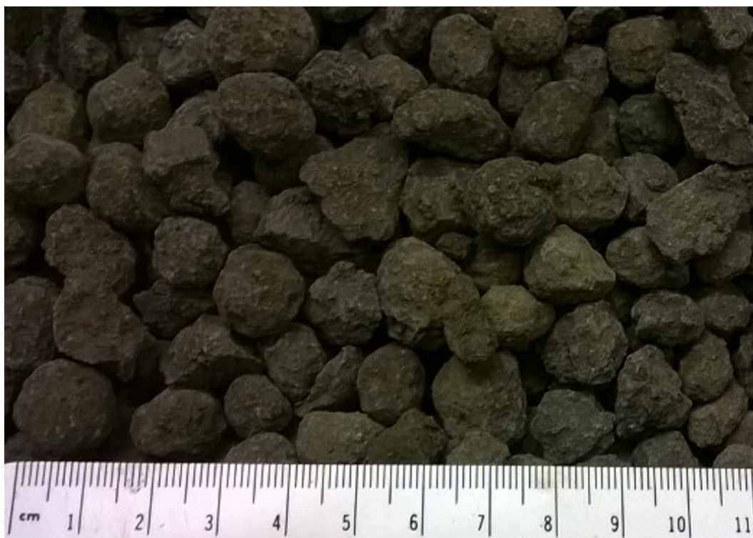
Fig. 1. As-received clinker sample ready for crushing and sieving
