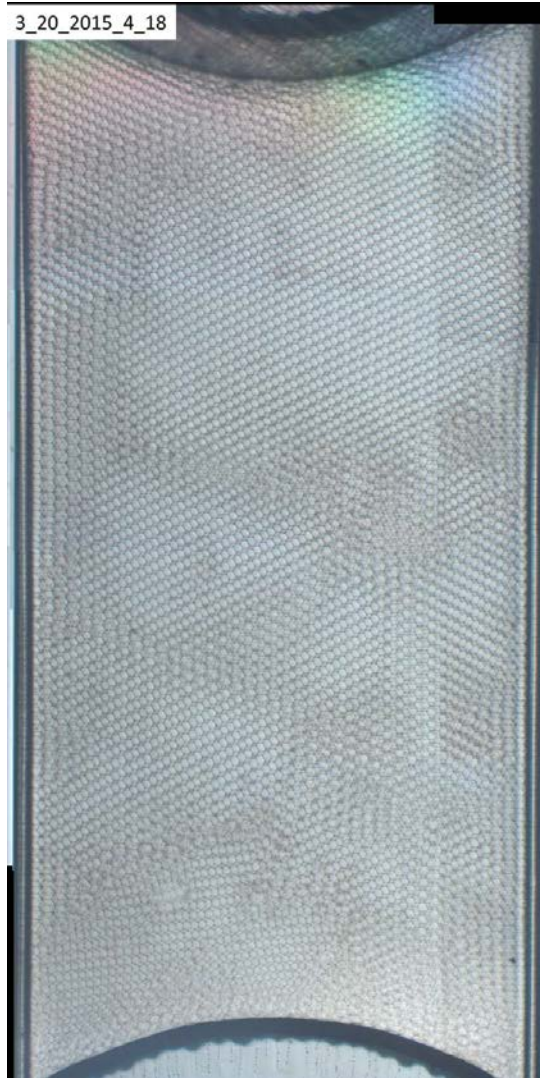
Figure 1: Emergence of lattice domain structure across a microfluidic plate. Channel dimensions ( L \times W \times H ) of the Ibidi #80621 \mu -Slide VI-flat hydrophobic are nominally 17 \text{ mm} \times 3.8 \text{ mm} \times 400 \text{ }\mu\text{m} . The mean diameter of the self-assembled aqueous emulsion droplets is on the order of 100 \text{ }\mu\text{m} .
