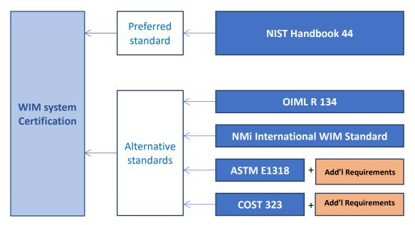
**Fig. 1.** Preferred and alternative standards to be used for certification of WIM systems. The application of ASTM E1318 and COST 323 may benefit from additional legal metrology requirements (see section 4.5).
