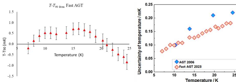
**Fig. 1.** Comparison of  $T-T_{90}$  for the Fast AGT thin lines, standard uncertainty of  $T-T_{90}$ ,  $u(T-T_{90})$ , the second graphic show  $u(T)$  for Fast AGT and AGT.
