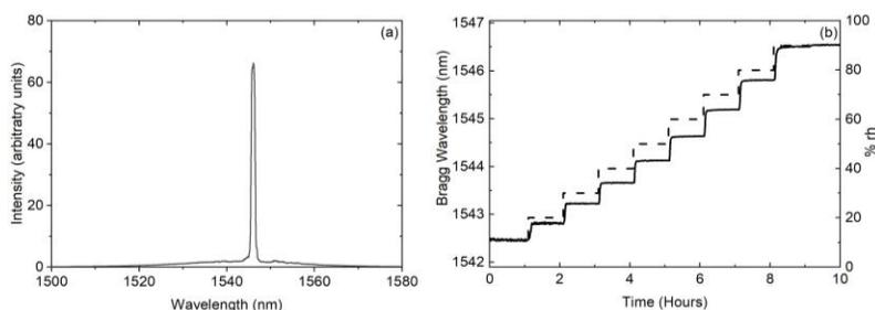
Figure 1 (a) Reflection spectra of the created grating. (b) Response of the grating (solid) to changes of relative humidity (dashed).
