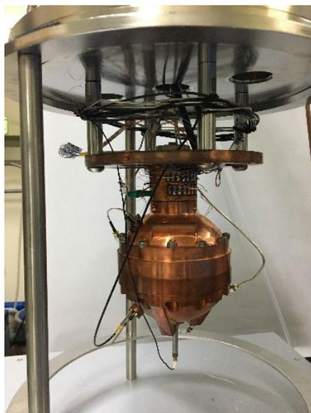
**Fig. 1.** The acoustic gas thermometer used in this work at KRISS.
