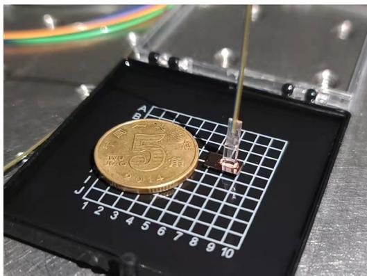
Fig.1 Packaged WGM photonic thermometer.
