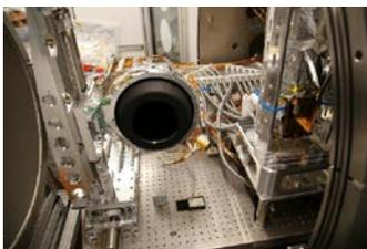
**Fig. 1. Photo of the RAL Space NGenIRS calibration target installed at the PTB facility.**
