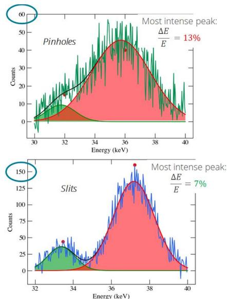
**Fig. 2.** Energy resolution quantification using Gaussian fitting of two GOS diffraction peaks.
