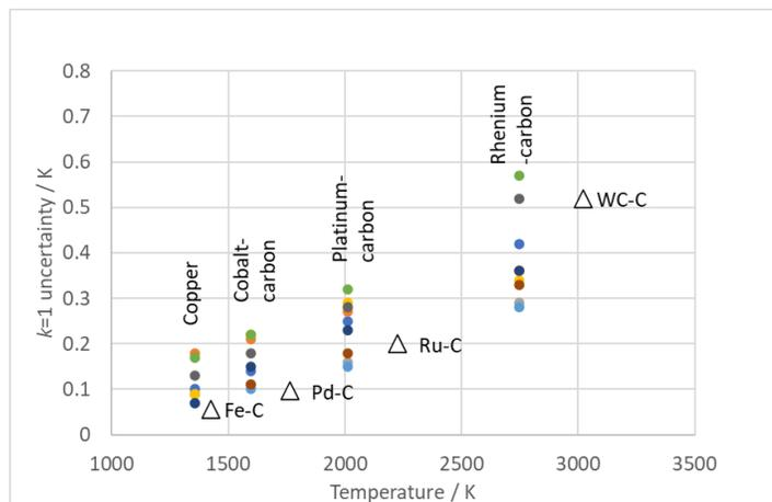
**Figure 1** Circles show previous state-of-the-art primary radiometry uncertainties at fixed points of Cu, Co-C, Pt-C and Re-C [4]. Triangles show the uncertainties achieved for relative primary radiometry at the fixed points of Fe-C, Pd-C, Ru-C and WC-C.
