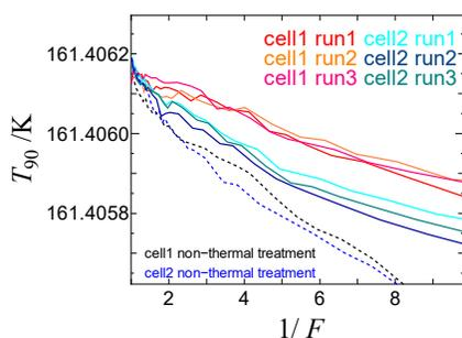
Fig. 1. Melting curves at the triple point of xenon.
