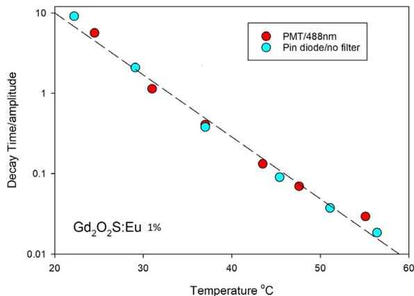
**Figure 2.** The parameter  $Q=[\text{decay time}/\text{amplitude}]$  versus temperature.
