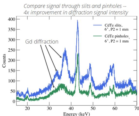
**Fig. 1.** Energy spectra of GOS:Tb showing both GOS diffraction peaks and x-ray fluorescence from gadolinium and tungsten. Slits (blue) attain better resolution and stronger signal than pinholes (green) as further demonstrated in Fig. 2.
