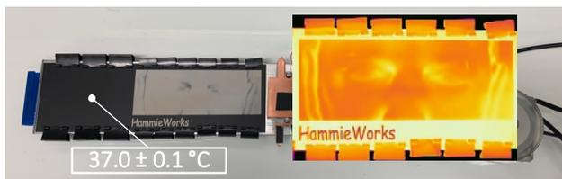
**Fig. 1.** A portable temperature-controlled heat pipe slab with a laser engraved facial thermograph image.
