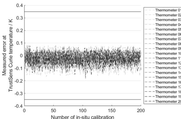
Fig. 2. Calibration data of 200 in situ calibrations of 20 thermometers
