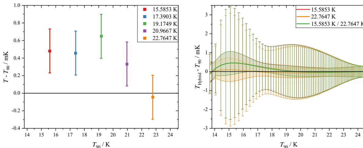
**Fig. 1.** Experimental determinations of  $T - T_{90}$  by AGT (left) and calculated “ $T_{\text{Hybrid}}$ ”-  $T_{90}$  differences (right); in the first case, only the uncertainty contribution from AGT is considered, while in the second one, this (lines with shaded areas) is compared with that of a typical  $T_{90}$  realization (error bars).
