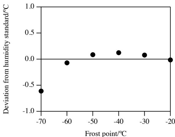
**Fig. 1.** Comparison with primary humidity standard.
