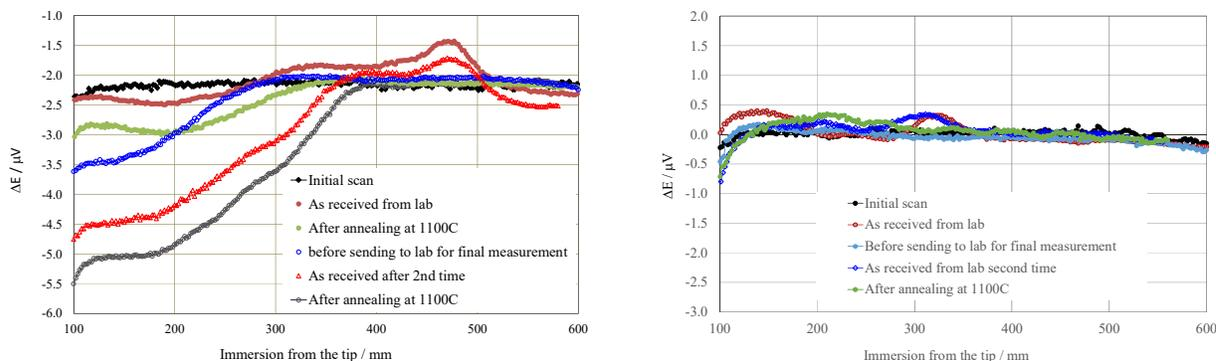
Fig 1. Typical inhomogeneity scans of two type R thermocouples in different stages of the comparison. Each thermocouple had been exposed to different calibration procedures.
