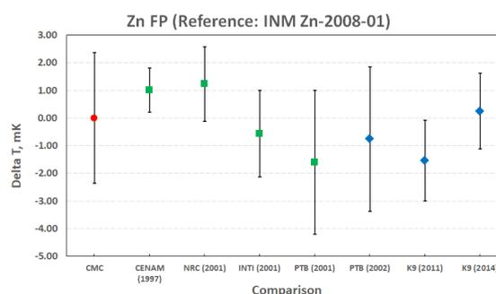
**Fig. 2.** Estimated comparison results if using Inmetro's reference Zn cell.
