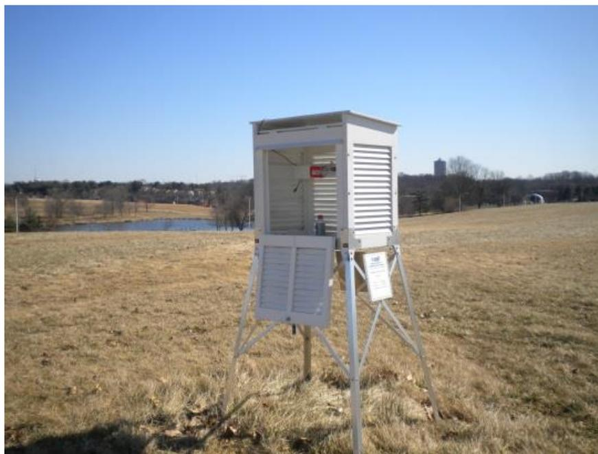
**Figure 1.** NIST Weather Box 1, Stevenson Shelter (shown with access door open).
