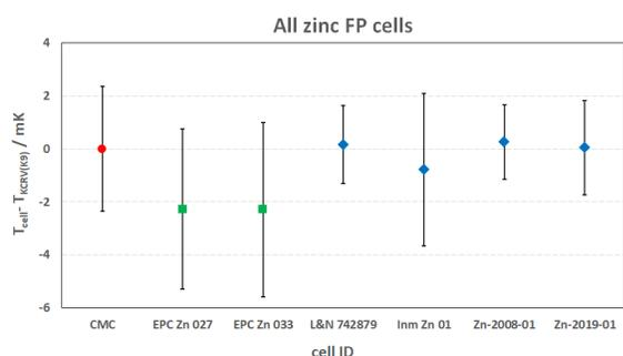
**Fig. 1.** Temperature differences and uncertainties for all Inmetro's Zn cells.
