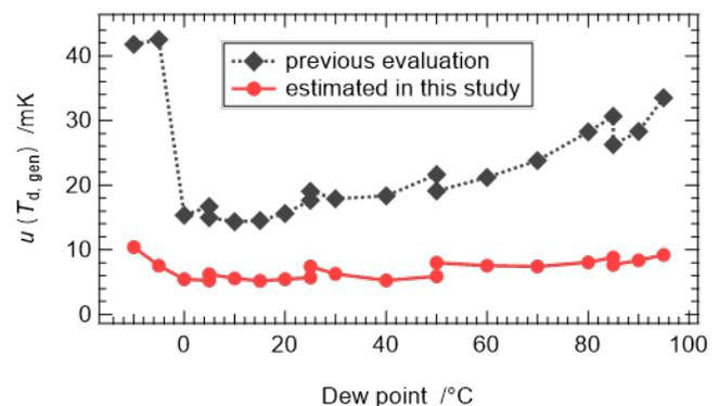
**Fig. 2. Combined standard uncertainty of generated dew-points  $u(T_{\text{d,gen}})$  estimated in this study (red) and the previous evaluation (black).**
