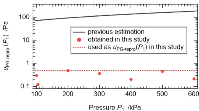
**Fig. 1. Standard uncertainty of reproducibility of the pressure gauge for saturator-pressure measurement  $u_{\text{PG-repro}}(P_1)$  obtained in this study (red) and the previous estimation (black).**
