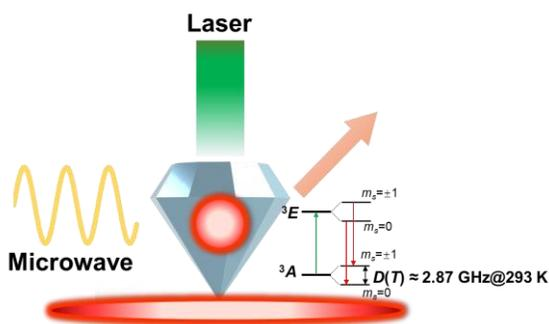
Fig.2. The schematic for NV in diamond thermometer
