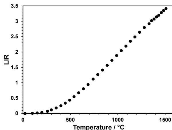
**Fig. 2.** Temperature dependence of measured Y<sub>2</sub>SiO<sub>5</sub>:Er area-averaged luminescence intensity ratio (LIR) (I<sub>488</sub>/I<sub>561</sub>) obtained from time-gated (1 μs) image.
