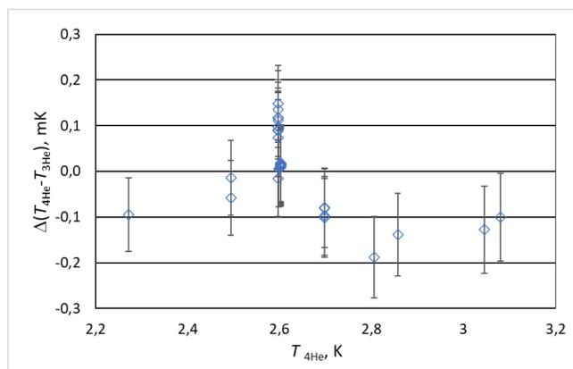
**Fig. 1. Results of the comparison between the  $^3\text{He}$  and  $^4\text{He}$  vapor pressure thermometers.**
