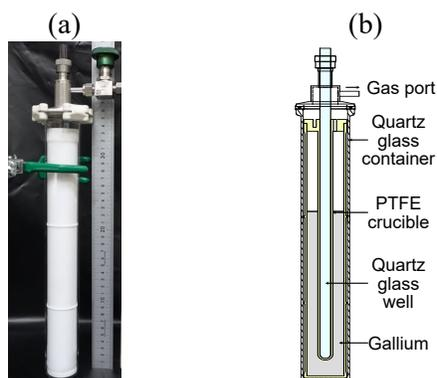
Fig. 1. Structure of the new gallium point cell.
