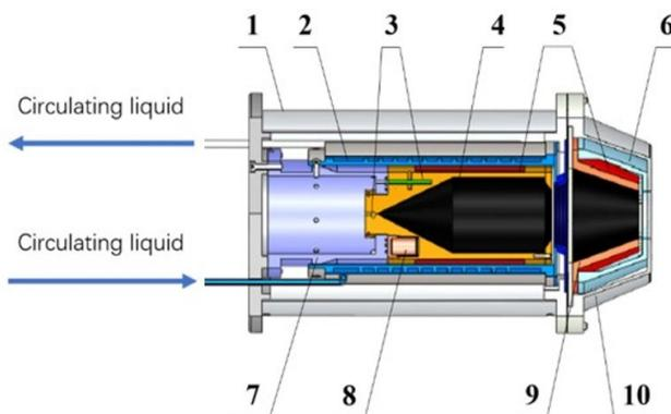
**Fig. 1.** Cross-sectional schematic of the spaceborne radiance temperature standard blackbody. 1-outer shield, 2-temperature control cover, 3-thermometer, 4-cavity, 5-heater, 6-insulation cover, 7-insulation structure, 8-MPFP, 9-TRL, 10- Outer shield
