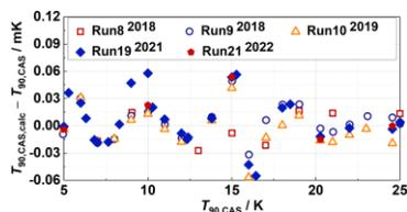
**Fig. 1.** The comparison results between  $T_{90,CAS,calc}$ , reproduced by the NIST calibrated RIRT from  $D(T_{NIST})$  equation, and the weight mean value  $T_{90,CAS}$ , experimentally determined the three RIRTs, in different runs of SPRIGT during 4 year.
