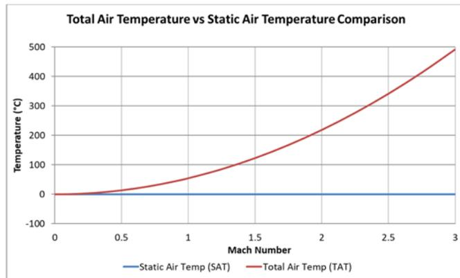
Fig. 1. TAT vs SAT Comparison.
