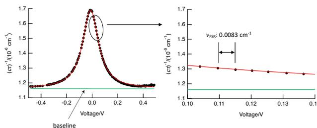
**Fig.1.** Absorption line of water in  $\text{N}_2$  obtained using the rapid-scan CRDS.
