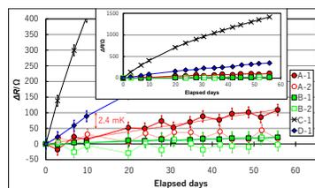
**Fig. 2.** Resistance changes of thermistors at the TPW.
