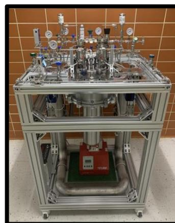
Figure 2. The noble triple point realization platform.
