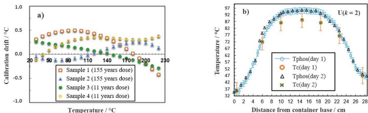
Fig 1. a) Phosphor thermometer calibration drift following exposure to ionizing radiation (Cf-252 – neutron); b) comparison of phosphor and thermocouple temperature measurements on a centrally heated dummy SNM container.
