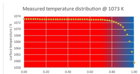
**Fig. 1.** Temperature distribution along the cavity wall of a sodium heat pipe blackbody at 1073 K obtained from radiometric measurements and iterative Monte-Carlo-Simulations.
