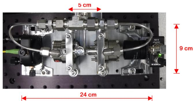
**Fig. 2.** Prototype of CRDS-based trace-moisture sensor [1].
