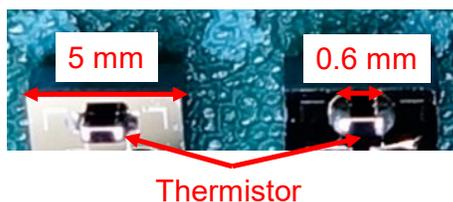
**Fig. 1.** Thermistors on silicon oxide substrates.
