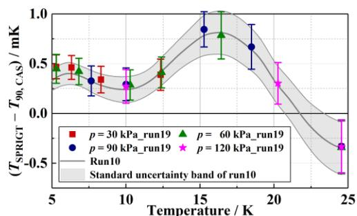
**Fig. 1.** Comparison of  $T-T_{90}$  for the SPRIGT method for two runs separated by an interval of 2.5 years. Lines: thick line,  $T-T_{90,CAS}$  determined in our previous work [2] (Table 9, run10); thin lines, standard uncertainty of  $T-T_{90,CAS}$ ,  $u(T-T_{90,CAS})$ . Symbols and error bars:  $T-T_{90,CAS}$  and  $u(T-T_{90,CAS})$  determined in the present work (run19) at different isobars (30, 60, 90, 120) kPa.
