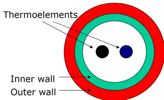
Fig. 1. Schematic drawing of a cross section of the dual wall thermocouple.
