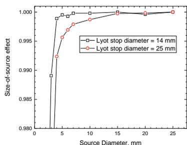
**Fig. 1.** SSE measured using two different Lyot-stop diameters.
