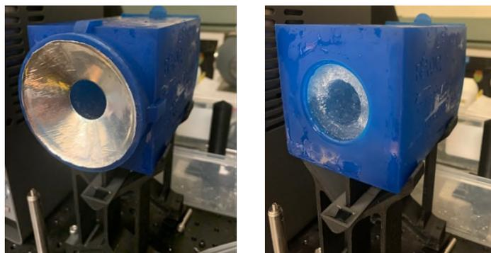
**Fig. 1.** The RADIP reference ice point in default configuration with well-defined diameter (left picture) using a reflective cone. When the cone is removed it reveals a controlled increase in diameter to determine dominant uncertainty (right picture).
