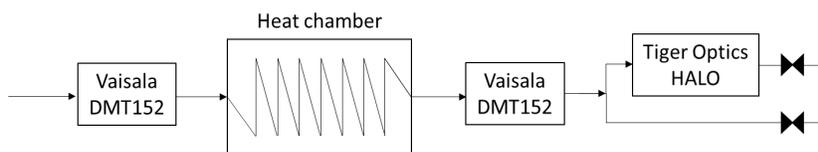
**Figure 1** Simplified measurement set-up. Unstable temperature of heat chamber causes adsorption or desorption. Trace moisture levels are measured by Vaisala’s DMT152 transmitters before and after a heat chamber along with a HALO from Tiger Optics.
