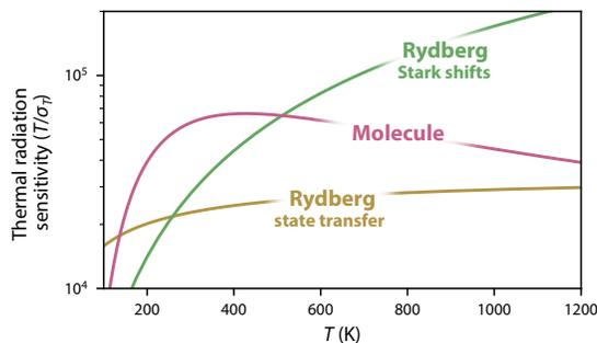
**Fig. 1.** Anticipated relative sensitivity, expressed in  $T/\sigma_T$  where  $\sigma_T$  is the anticipated 1 standard-deviation statistical uncertainty of a measurement with  $10^9$  atoms or molecules, of different blackbody radiation sensors as a function of temperature  $T$ . Figured adapted from Ref. [1].
