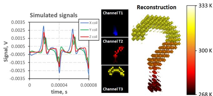
**Fig. 1.** 20x20x20 voxels 3D temperature image reconstruction process.
