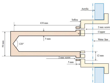
**Fig. 1.** Reference blackbody cavity design.
