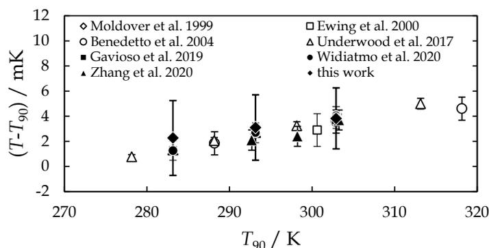
Fig. 1. Available  $(T-T_{90})$  from AGT and the present result.
