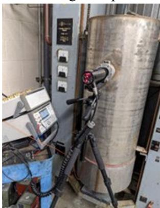
**Fig. 1.** Spectra-mat furnace with optical pyrometer, thermocouples, and data logger.
