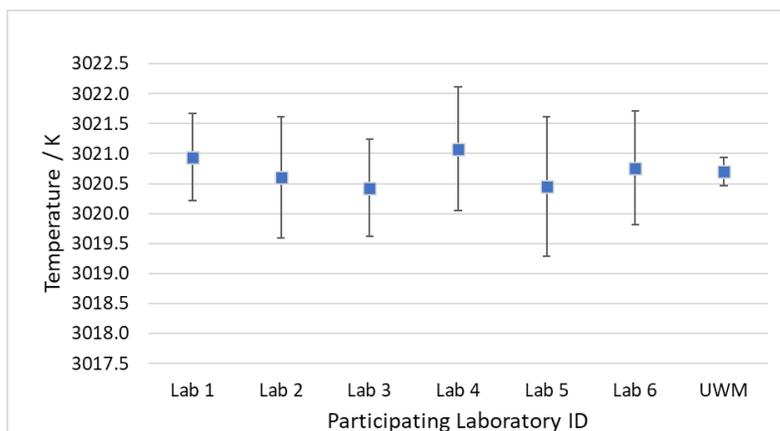
**Fig. 1.** Reported point-of-inflection thermodynamic temperatures and uncertainties ( $k=2$ ) from participating laboratories, compared to the uncertainty-weighted mean (UWM) with its uncertainty (including thermal effects)
