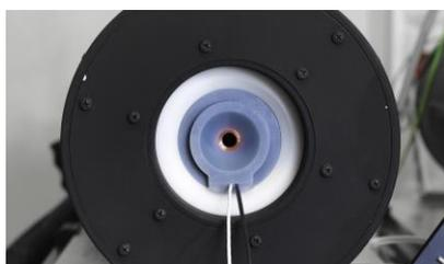
**Fig. 2.** Photograph of the ammonia-heatpipe equipped with the tempered aperture.
