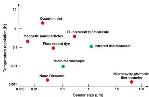
Fig. 1. The resolution for different methods
