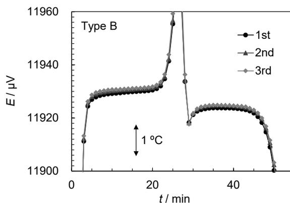
Fig. 1. The melting and freezing curves of Rh-C alloy.
