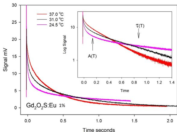
**Figure 1.** Luminescence signal versus time at 24.5, 31, and 37.0 °C. The inset is a semilog plot of the same. Detector: PMT with 488 nm bandpass filter.
