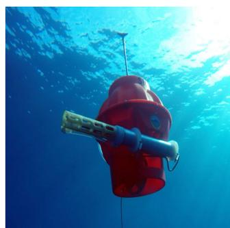
**Fig. 2.** Deep Argo, a new type of Argo float capable of sampling from the surface to 6 km, with the more accurate SBE 61 CTD. Image from [4]
