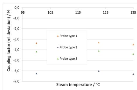
**Fig. 2. Measurement error of different probe types at various steam temperatures**
