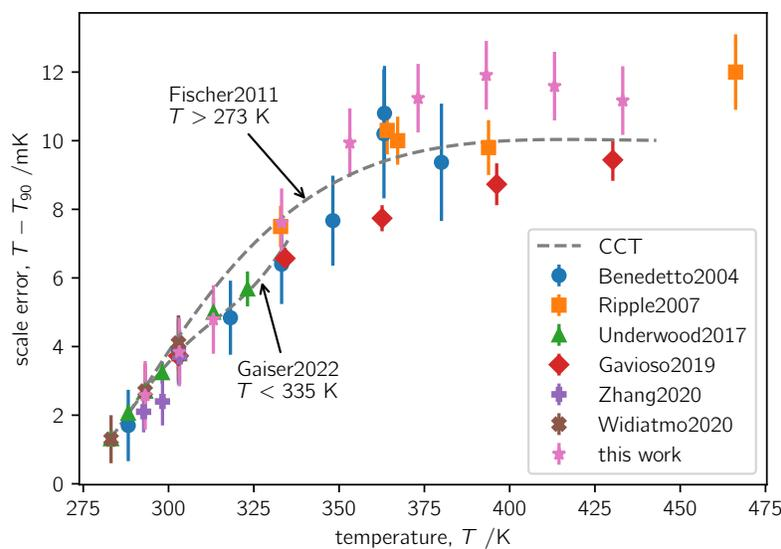
**Fig. 1.** Measurements of the scale error in ITS-90.
