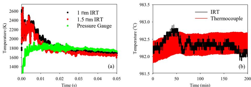
**Fig. 1.** (a) Confined blast load IRT temperature measurement in comparison to pressure gauge and (b) high temperature sapphire-based FO-IRT target temperature drift measurement in comparison to thermocouple.
