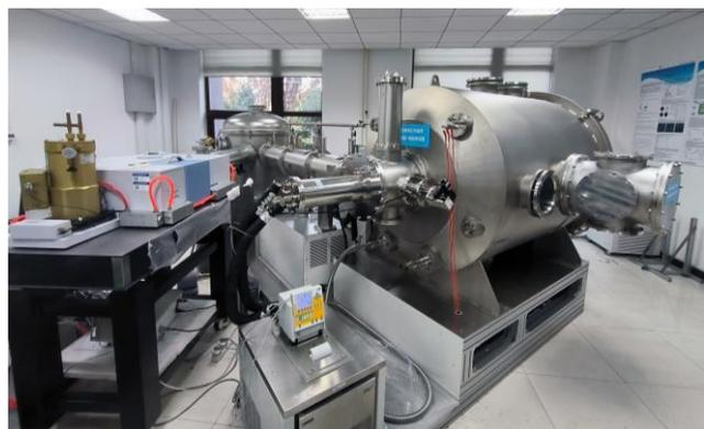
**Fig. 1.** The new generation of Vacuum Infrared Radiance Temperature Standard Facility.
