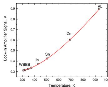
**Fig. 2.** Measurements performed using a variable-temperature BB to demonstrate the range in operational temperatures. A Sakuma-Planck interpolation function fit is shown.
