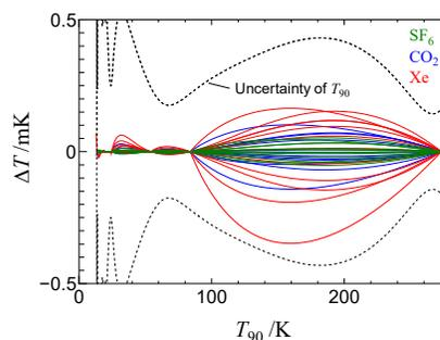
Fig. 2. The temperature difference  $T_{XX}-T_{90}$  (XX is SF<sub>6</sub>, CO<sub>2</sub> or Xe) of SPRTs with four subranges.
