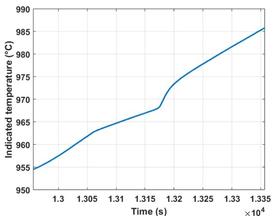
**Fig. 1.** Melting curve with plateau using a silver ingot.
