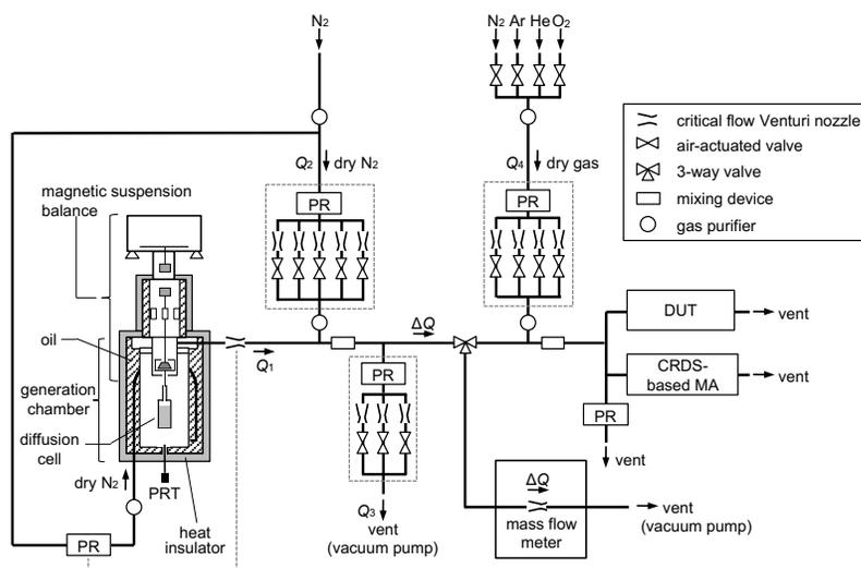
Fig.1. Schematic of the Multi-gas Trace-moisture Generator
