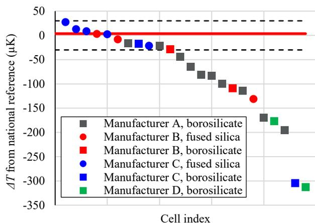
**Fig. 1.** Measured temperature difference of the triple-point-of-water cells from the national reference of KRISS.
