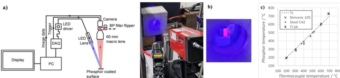
**Fig. 1.** Imaging intensity ratio phosphor thermometer: a) design scheme, b) measurements on an induction furnace, and c) phosphor temperature versus embedded thermocouple for three different engineering alloys.
