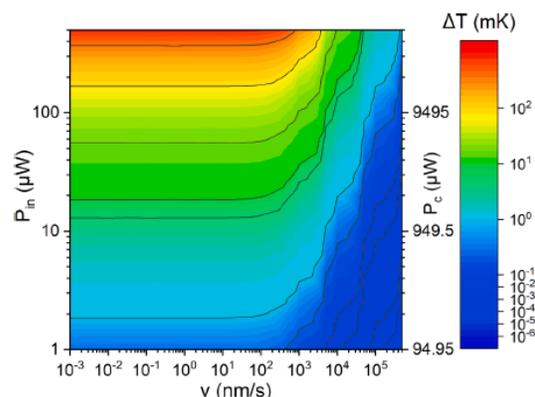
Fig.2 Prediction of the self-heating temperature rise.
