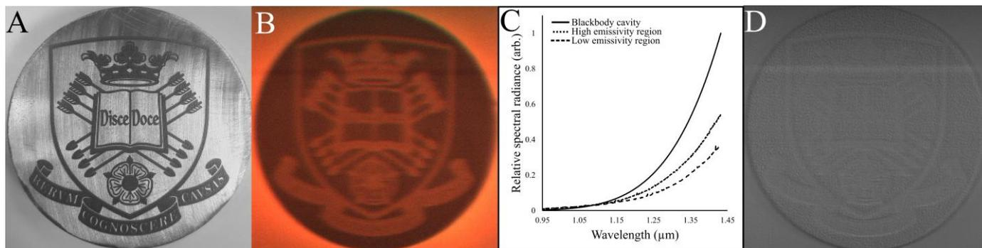
Figure 1 (A) A photograph of a laser etched target; (B) A pseudo RGB image of the target heated to 378 °C; (C) A plot of relative spectral radiance against wavelength; (D) A ratio of the images corresponding to 1.33 and 1.43  $\mu\text{m}$ .
