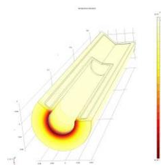
**Fig. 2.** Temperature distribution of a sodium heatpipe at 1073 K, calculated using an FEM simulation.
