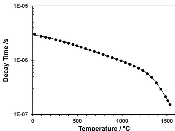
**Fig. 1.** Temperature dependence of Y<sub>2</sub>SiO<sub>5</sub>:Er decay time from furnace calibration measurements. Excitation at 522 nm, emission detected at 542 nm.
