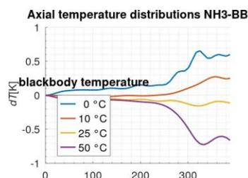
**Fig. 1.** Measured axial temperature profiles [2] of the ammonia-heatpipe blackbody w/o aperture.
