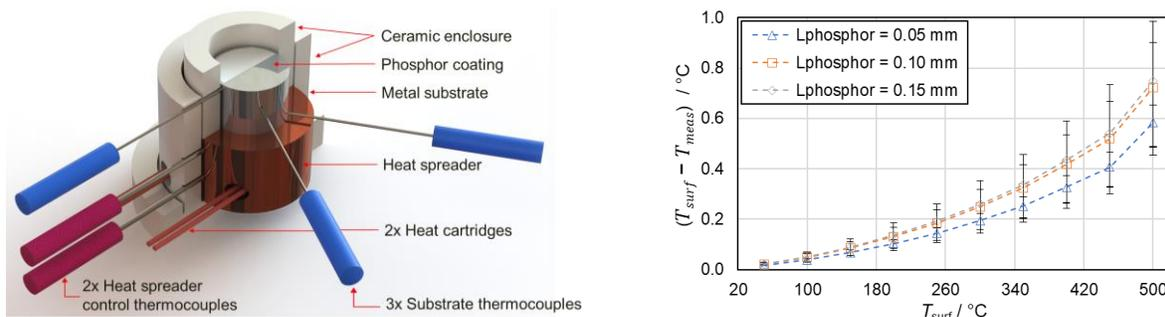
**Fig. 1.** Left. Design of the phosphor calibration system. Right. Calculated difference ( $T_{surf} - T_{meas}$ ) for three coating thicknesses, for temperatures up to  $500 \text{ }^\circ\text{C}$ . The error bars represent the change in values for a  $1 \sigma$  change of  $\Delta = \pm 0.017 \text{ mm}$  (coating thickness).
