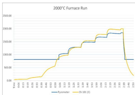
**Fig. 2.** Optical pyrometer (blue) versus thermocouple data (yellow) for a nominally 2000°C run.
