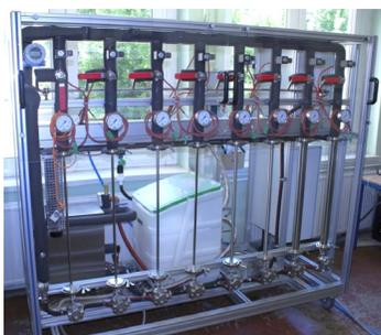
**Fig. 1. Test bench for investigation of pipe clamp probes**
