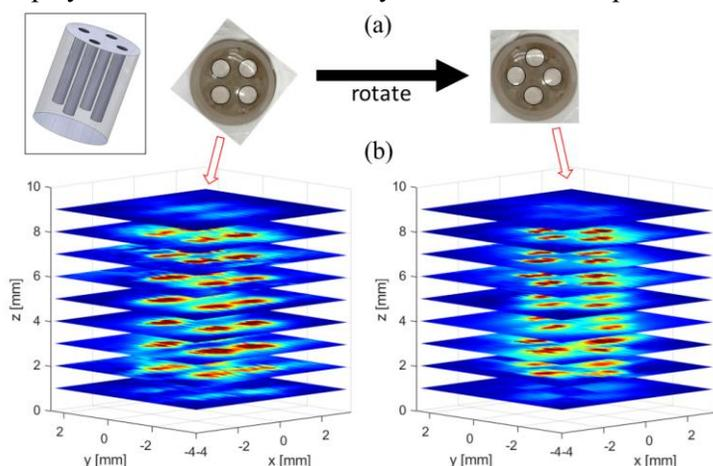
Figure 1: 3D MPI image (b) of magnetic nanoparticles embedded in a 4 channel glass phantom (a).
