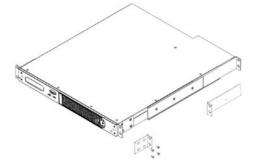
2. Mount the appliance in the equipment rack. Alternatively, ignore the rails and mounting tabs, and rest the Luna SA appliance on a mounting tray or shelf suitable for the organization's specific style and brand of equipment rack.
