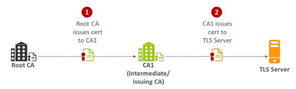
As shown in Figure 2-7, when a client, such as a browser, connects to a TLS server, the server will return its certificate as well as the certificate for the CA that issued its certificate (called the CA certificate chain).
