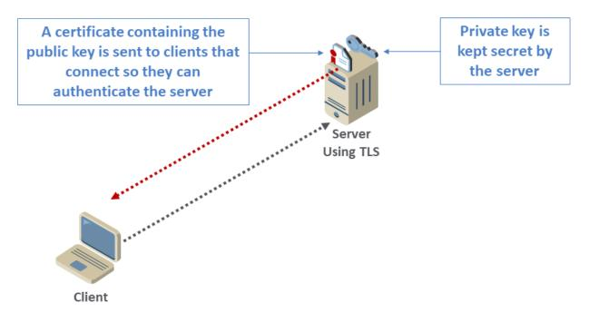
In addition to users with browsers connecting to servers that have TLS server certificates, automated processes also connect as clients to TLS servers and must trust TLS server certificates. Examples of automated processes acting as TLS clients include a web server making requests to an application server, one cloud container connecting to another, or an Internet of Things (IoT) device connecting to a cloud service. (See Figure 2-4.)
