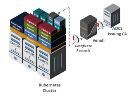
Figure 4-5 Example Implementation's DevOps Components Requesting and Receiving Certificates
