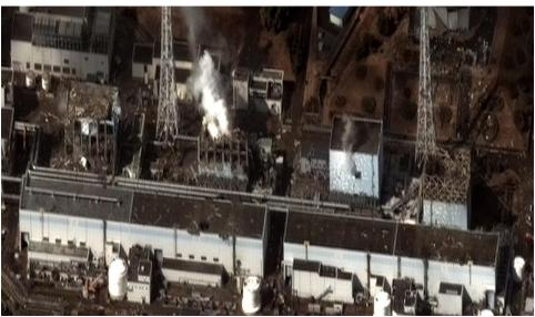
Figure 2 (a). Fukushima Daiichi nuclear disaster, 16 March 2011, showing the four tall damaged reactor buildings with much of the damage caused by hydrogen—air explosions, Fukushima, Japan Source: <a href="https://en.wikipedia.org/">https://en.wikipedia.org/</a>
