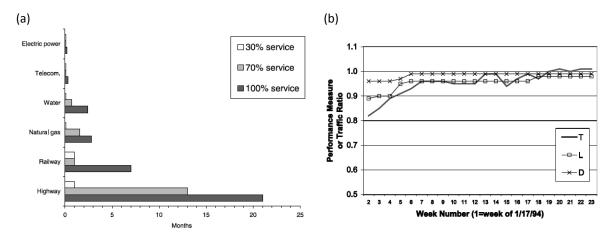
Figure 1. Infrastructure restoration curves. (a) for different systems in 1995 Kobe earthquake, (b) according to different service measures (T, L, D) for highway transport service in the 1994 Northridge earthquake. (source: Chang and Nojima, 2001)
