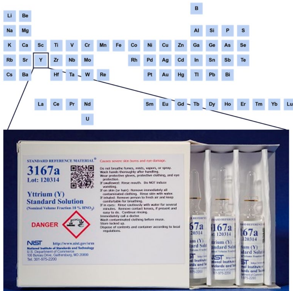
Figure 10: (Top) The single-element standards included in the NIST SRM 3100 series encompass a range of CMMs indicated by the blue elements. (Bottom) NIST SRM 3167a, Yttrium (Y) standard solution, part of the 3100 series, is used to quantify CMMs across various materials, serving applications from basic research to quality assurance and quality control in industrial production. Credit: NIST.
