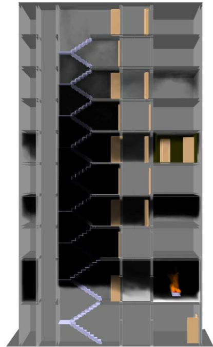
Smokeview rendition of the smoke in a Fire Dynamics Simulator (FDS) simulation of a fire in a multi-story building. (Credit: NIST)
