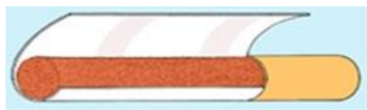
Schematic of a cigarette showing the bands in the wrapping paper to slow burning rate. (Credit: NIST)
