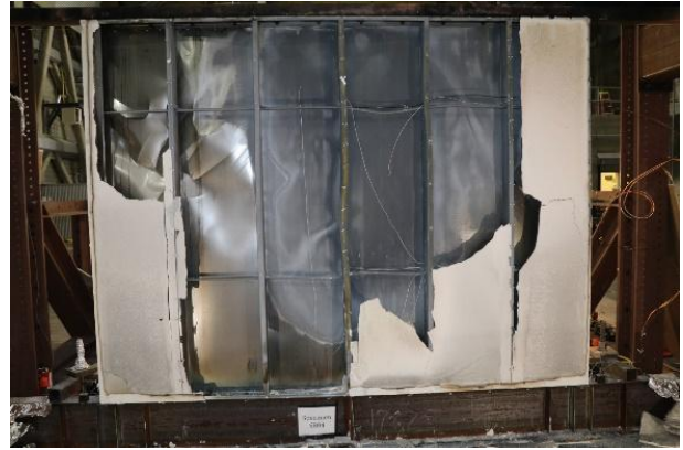
Result of a test of a steel wall under earthquake and fire conditions. (Credit: NIST)
