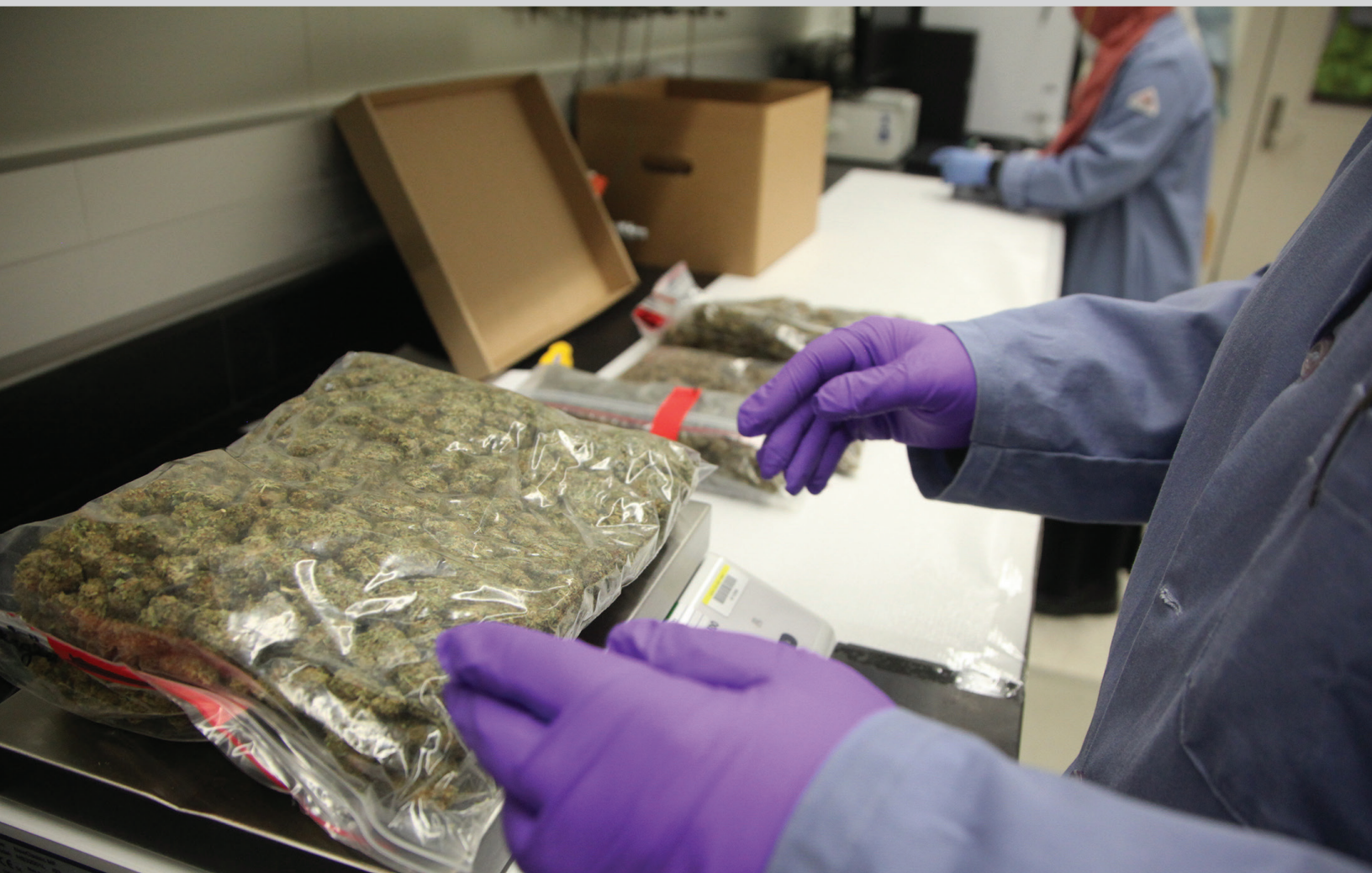
NIST researchers weigh packages of marijuana prior to preparing samples with very precisely measured amounts of tetrahydrocannabinol (THC), cannabidiol (CBD), and other compounds. Those samples were then sent to labs as part of an interlaboratory study to help labs improve their measurement accuracy.
