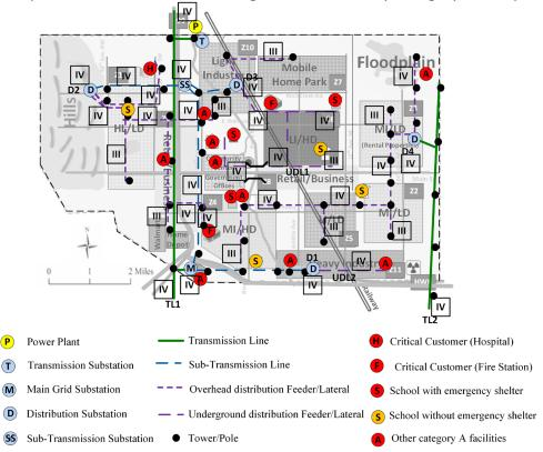
Fig. 5-5. Electric power grid components assigned Criticality Categories.
