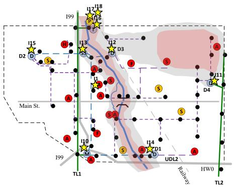
**Fig. 5-8.** General extent and severity of damage to power grid components in Centerville caused by the earthquake. Shaded areas represent in a qualitative way ground motion and permanent ground deformation decreasing from the river and Centerville's flood plain. Yellow star identifies a damage location. See also legend in Fig. 5-6.
