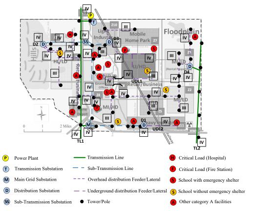
Fig. 5-3. Centerville electric power grid and assigned Criticality Categories.
