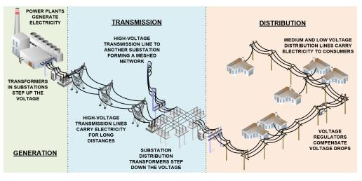
Fig. 5-1. Simplified representation of the three subsystems forming an electric power system.
