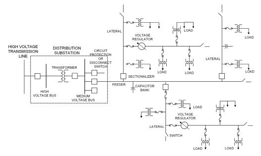
**Fig. 5-2.** Representation of part of a typical electric power distribution subsystem. Electric power flows from left to right.
