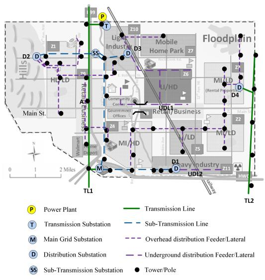
Fig. 2-5. Centerville electric power system (gray shaded base map modified from Ellingwood et al. [2016]).
