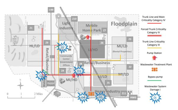
Fig. 4-2 Centerville wastewater system damage locations.
