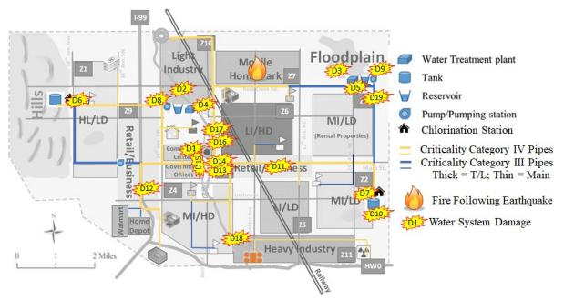
Fig. 3-2. Centerville water system damage locations, except for the water distribution pipelines leaks and breaks.
