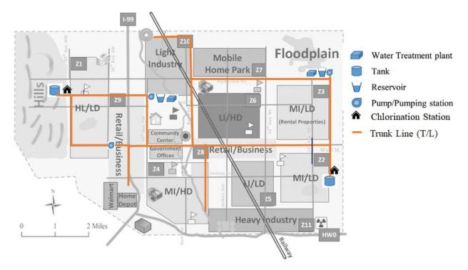
Fig. 2-3. Centerville potable water system (gray shaded base map modified from Ellingwood et al. [2016]).
