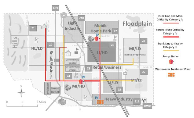
Fig. 4-1. Centerville wastewater system layout and assigned component Criticality Categories.
