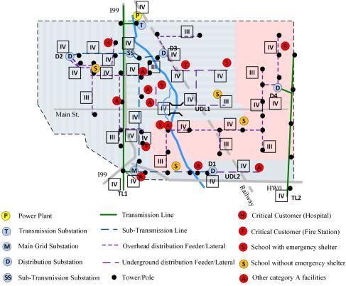
Fig. 5-6. Service area for each transmission line and each distribution substation in Centerville. Component Criticality Categories are identified.
