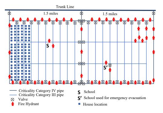
**Fig. A-1.** Example potable water distribution pipe grid (4.82 km by 2.78 km or 3 miles by 1.5 miles). For clarity, not all houses or fire hydrants are shown.
