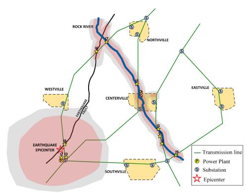
**Fig. 5-7.** General extent and severity of damage to power grid components at a regional level. Shaded areas represent in a qualitative way ground motion and permanent ground deformation decreasing from the epicenter, the river and Centerville's flood plain. Yellow star identifies a damage location.
