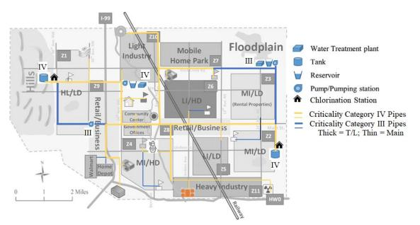
Fig. 3-1. Centerville water system layout and assigned component Criticality Categories.
