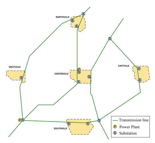
Fig. 2-6. Electric power transmission grid in the region around Centerville.
