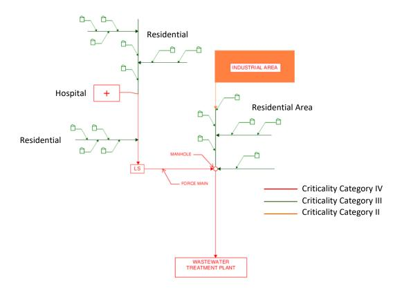
Fig. A-2. Example wastewater pipe network.
