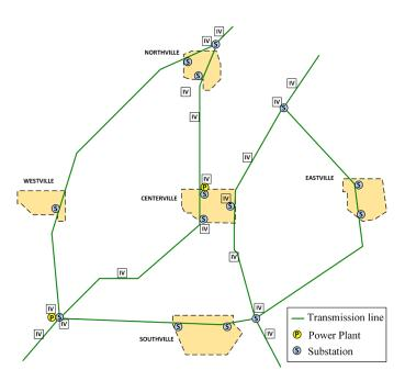
Fig. 5-4. Electric power grid in region around Centerville. Criticality Categories are only indicated from Centerville's perspective.
