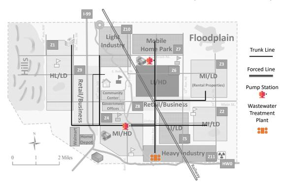
Fig. 2-4. Centerville wastewater system (gray shaded base map modified from Ellingwood et al. [2016]).
