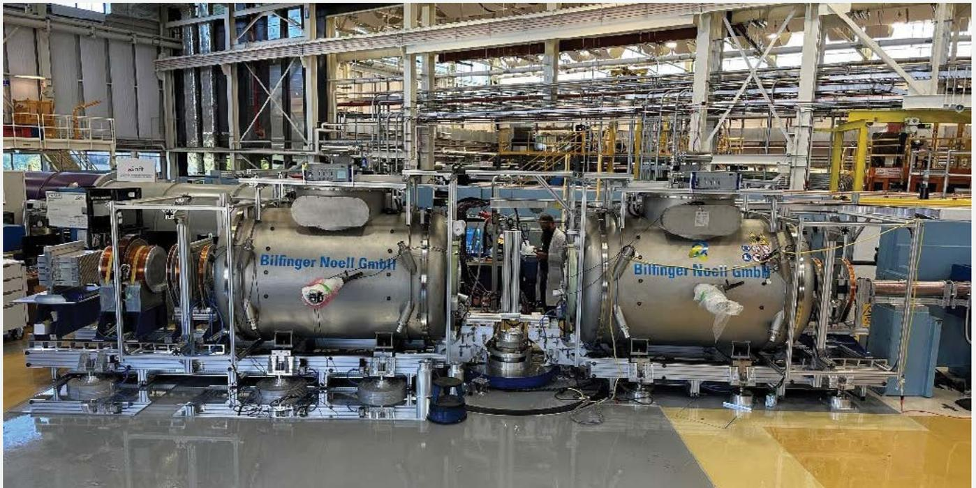
**FIGURE 2:** v-NSE in Fall 2023, with superconducting coils and epoxy airpad dancefloor in place.
