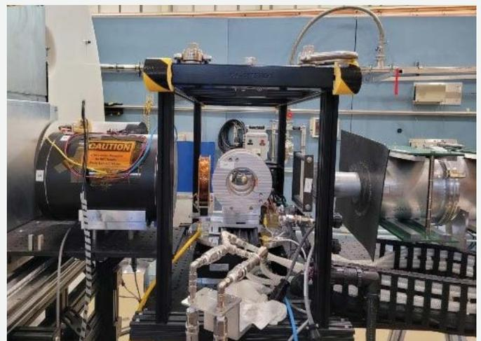
**FIGURE 4:** Low-field setup for full-polarization measurements at vSANS. Photo at top corresponds to sample field parallel to the beam direction, at bottom is for field perpendicular.
