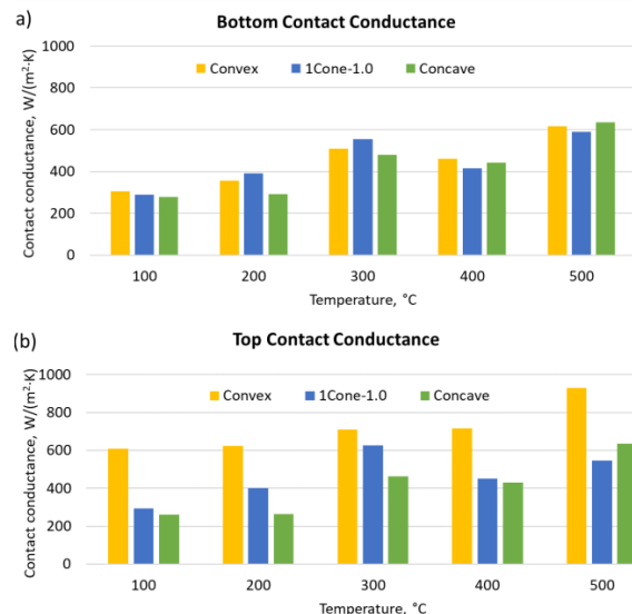
FIGURE 10: SIMULATED CONTACT CONDUCTANCE (A) AT THE BOTTOM, AND (B) ON THE TOP OF THE INTERNAL POWDER AND SOLID SHELL
