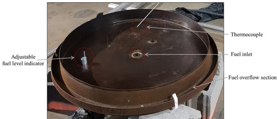
Fig. 1. The 1 m diameter, water-cooled, round steel burner with fuel level indicator and fuel overflow section. The S type thermocouple used to measure the gas phase temperature is also shown.
