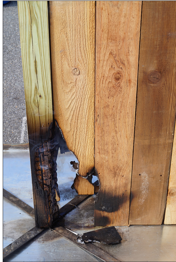
Figure 14 —Parallel western redcedar privacy fences without mulch at low wind speed (6 m second -1 ).
