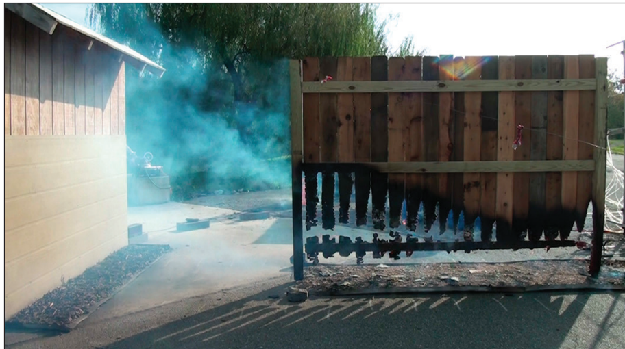
Figure 12 —Single western redcedar privacy fence in hardwood mulch at low wind speed ( 6 \text{ m second}^{-1} ).
