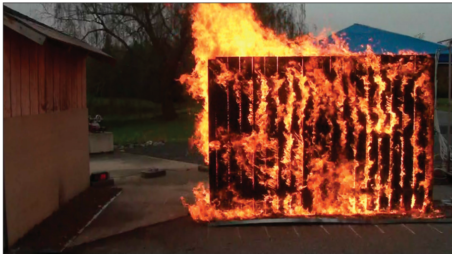
Figure 13 —Parallel western redcedar privacy fences separated by 0.20 m in hardwood mulch at low wind speed ( 6 \text{ m second}^{-1} ).
