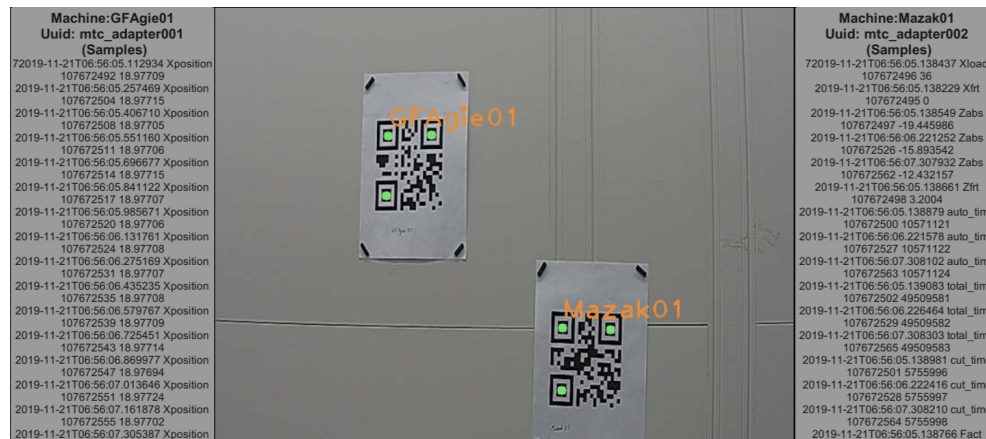
Figure 2: Real-time MTConnect data is shown for the detected machines.
