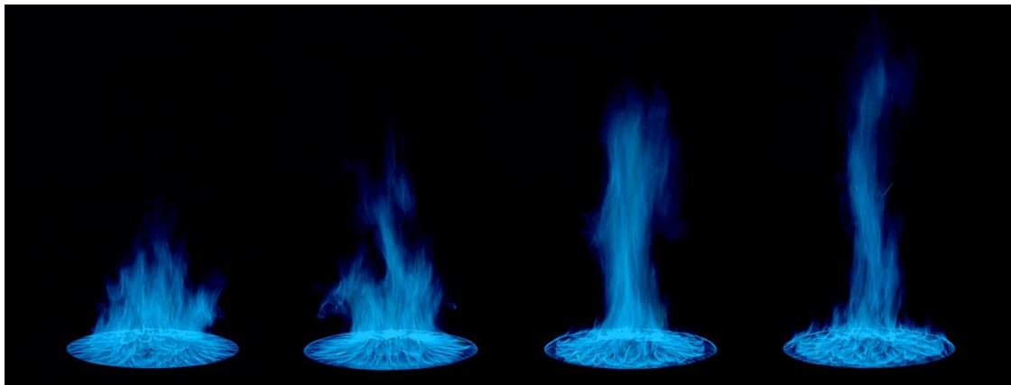
Fig. 4. Instantaneous digital images 132 ms apart in the pulsing 1 m diameter methanol pool fire.
