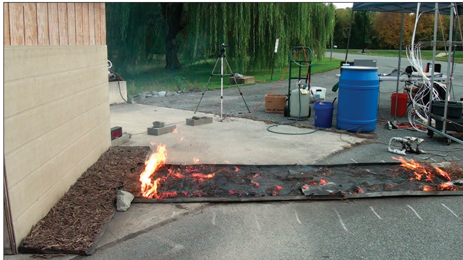
Figure 15 —Pine straw mulch bed in contact with target hardwood mulch bed.
