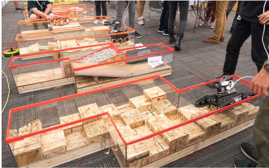
Figure 2: Terrain test method apparatuses arranged as individual lanes for preliminary trials.
