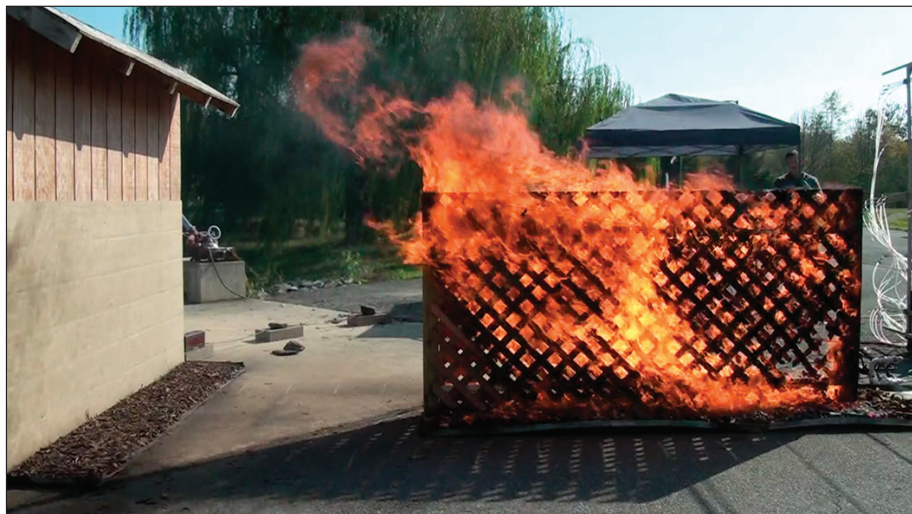
Figure 10 —Double redwood lattice fence in hardwood mulch at low wind speed ( 6 \text{ m second}^{-1} ).
