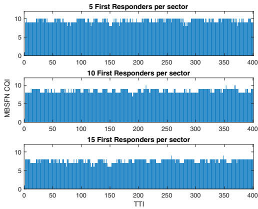
Fig. 11: MBSFN Minimum CQI with Time
