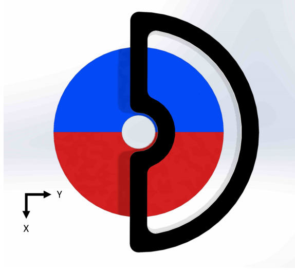
Fig. 3. Top view of magnet assembly where the upper magnet and encoder scale are hidden for clarity to show D-Coil. This orientation represents where \theta_{z'} = 0 .
