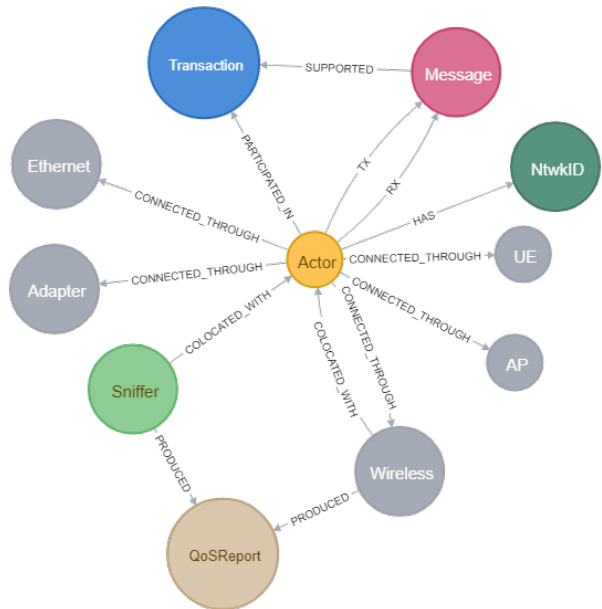
Fig. 4: Realized schema of the graph database fully populated after capturing network and operational data from the NIST industrial wireless testbed.
