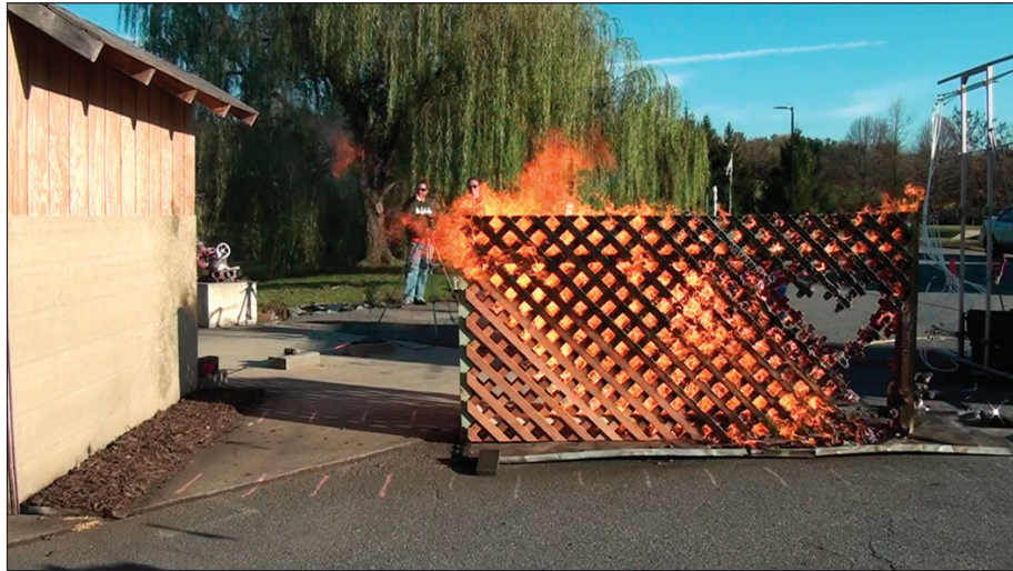
Figure 11 —Double redwood lattice fence without mulch at low wind speed ( 6 \text{ m second}^{-1} ).
