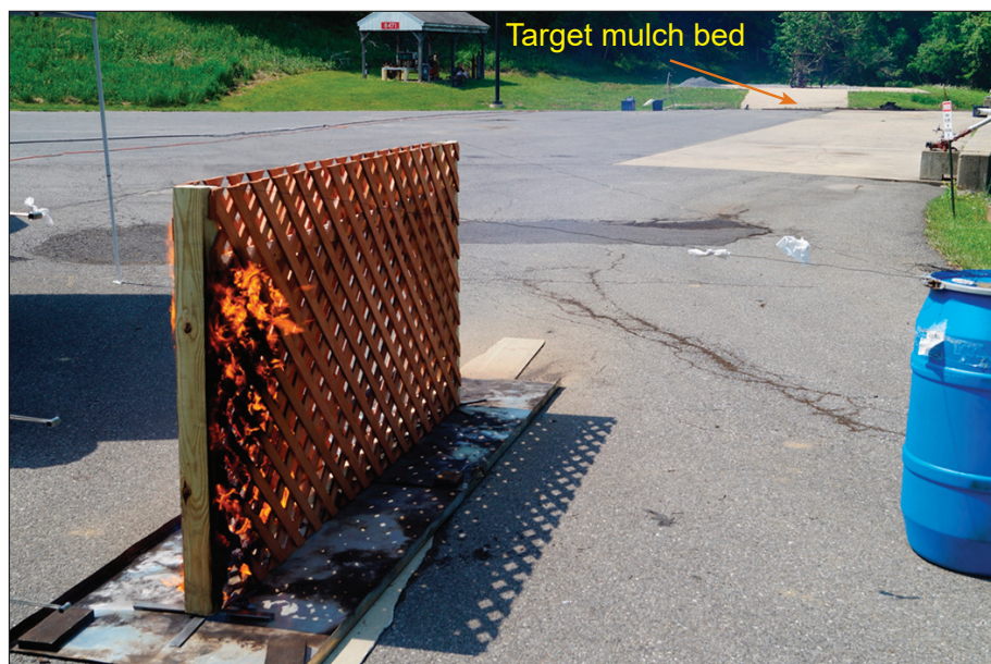
Figure 16 —Double lattice fence experiment without a structure and with a mulch bed situated 23 m from the far end of the fence.
