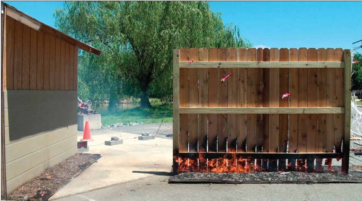
Figure 3 —Image from video of western redcedar fence combined with shredded hardwood mulch.
