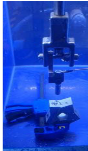
FIG. 13 CUT side inspection of the aluminum star artifact.
