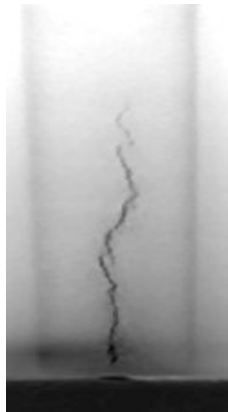
FIG. 38 Organic defect (hot tear or crack) in Region 2.
