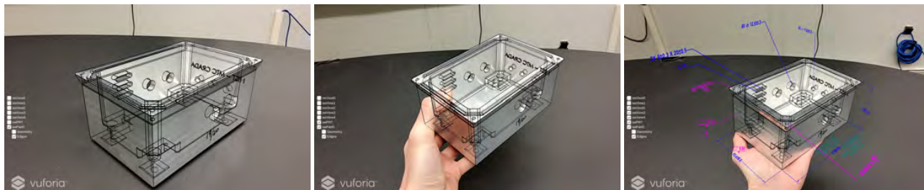
Figure 5: AR view of the wire-frame of the part geometry overlaid on the physical part.
