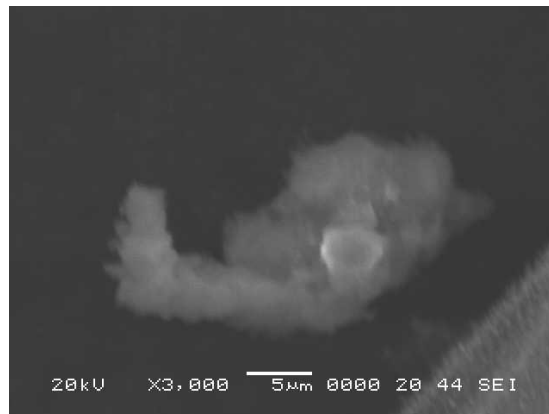
Figure 4 SEM image of soot agglomerate with a grid insertion time of 3 sec.
