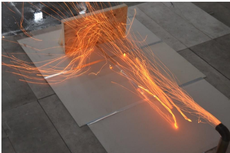
Figure 3 As an example of the physics involved, showers of laboratory generated firebrands combusting in a wind field of 8 m/s are directed at a simplified flow obstruction of 660 cm (H) by 1275 cm (W) obstacle. Here, Japanese Cypress wood chips are used as the source of firebrands.
