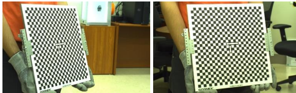
Figure 11. One pair of images from left and right cameras used for stereo calibration
