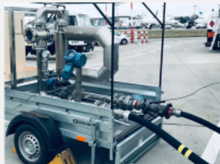
Evaluating field reference meters for traceability of transportation fuels
