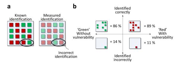
**Figure 6.** (a) Example of a map of known identification and a map of measured identification. We deliberately chose unequal totals for the number of red and green circuits. The example includes 2 incorrectly identified devices. (b) A quadrant chart showing the correct and incorrect identifications for the red and green devices.
