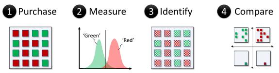
**Figure 7.** Measurement verification process. A user obtains a standard test article that they measure with one or more measurement techniques. Then, a classification step groups circuits into 'red' and 'green' classes. The next step compares the measured identification to the known identification, which produces metrics that can quantify the performance of the measurement technique against alternative measurement-based approaches.
