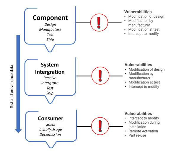
**Figure 3.** A high-level view of some hardware security vulnerabilities in the supply chain of a completed system, such as a cell phone, gNB, or 5G enabled vehicle. Each step in the supply chain has unique vulnerabilities. A comprehensive security strategy needs to address the unique aspects of each step in the chain and consider the use case, risk, and cost of mitigation actions (adapted from [145]).
