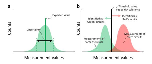
**Figure 5.** (a) Example of a distribution of measurement values. (b) Example of two distributions of measurements of a hypothetical standard test article that includes 'green' circuits without a vulnerability and 'red' circuits with a vulnerability. In this case, a threshold value is a hard cutoff used to identify both the 'red' and 'green' circuits.
