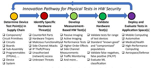
Figure 8. Innovation pathway for developing physical tests for hardware security.
