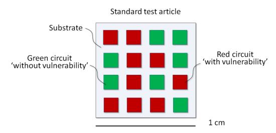
**Figure 4.** Example of a standard test article for quantifying a measurement techniques' ability to measure specific vulnerabilities. This standard test article allows comparisons across disparate measurement modalities that otherwise produce measurements that cannot be compared directly.
