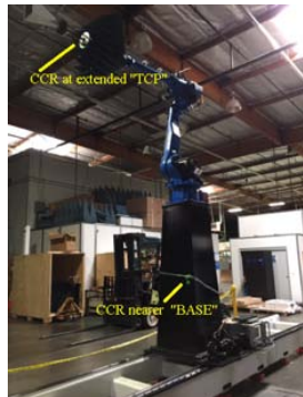
Figure 11. Positions of the laser tracker targets on the MR base and TCP to measure cross range movement while the MR is moving.
