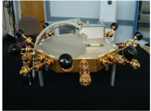
Figure 1: Custom-designed 16-port octagonal receiver antenna array.
