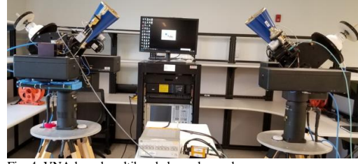
Fig. 4: VNA-based multiband channel sounder.
