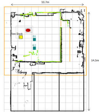
Figure 3. Room floor plan made by navigation system with 1 m grid lines. The red circle indicates the robot position.
