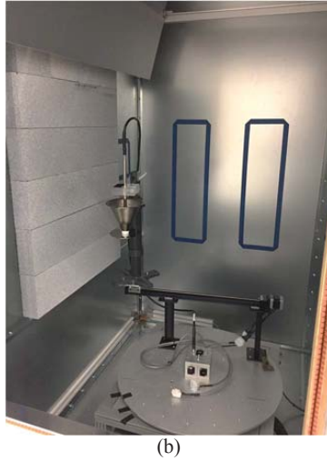
Fig. 1. Experimental setup for synthetic-aperture measurements: (a) top-down diagram and (b) photograph of chamber with loaded wall at left.
