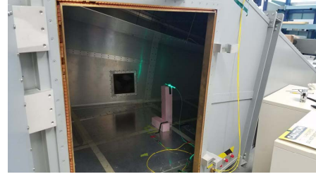
Fig. 5: Fiber-probe inside a GTEM cell.
