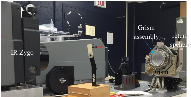
Figure 20. Test layout of the grism assembly in front of an IR interferometer with a flag indicating the focus position of the transmission sphere.
