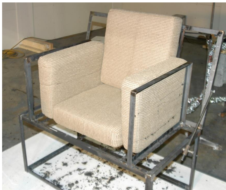
Figure 3. Photograph showing four cushions in place on the test stand.
