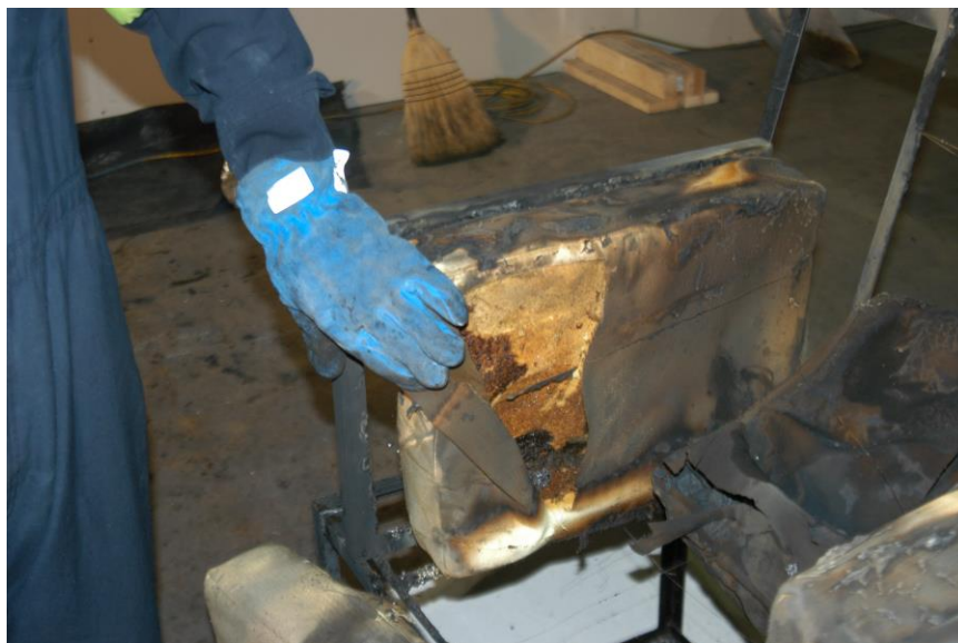
Figure 116. Images showing the remaining charred material on the mock-up stand following Test 22_2. The seat cushion has been removed, and the Norfab fabric on the left arm has been cut to expose the FRFPUF underneath. The partially collapsed back cushion is located to the right of the arm cushion.
