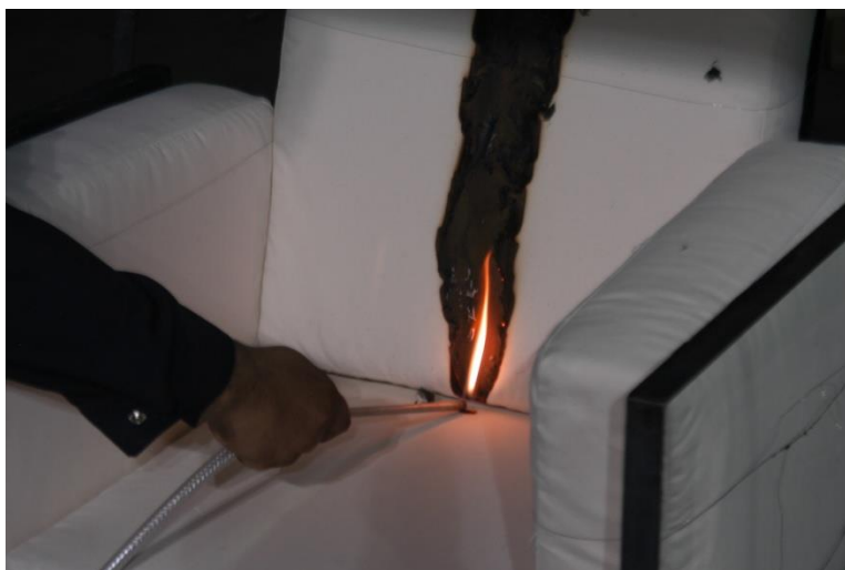
Figure 14. Photograph showing ignition of a furniture mock-up with Ignition Source 2.
