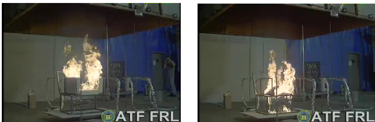
Figure 30. Two frames taken from a video recorded by Camera #8 show the appearance of the fire during Test 9_1 at 401 s (left) and 544 s (right) following application of Ignition Source 1.
