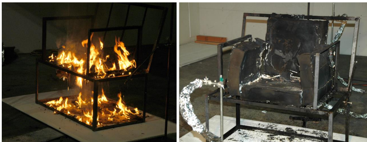
Figure 68 Photographs showing mock-ups during Test 14_1 as it was burning out (left) and Test 25_1 (right) after the flames had extinguished.
