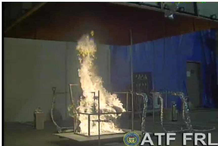
Figure 112. A frame taken from a video recorded by Camera #8 672 s following ignition shows the fire burning on the test stand base and the remaining mock-up during Test 20_1.
