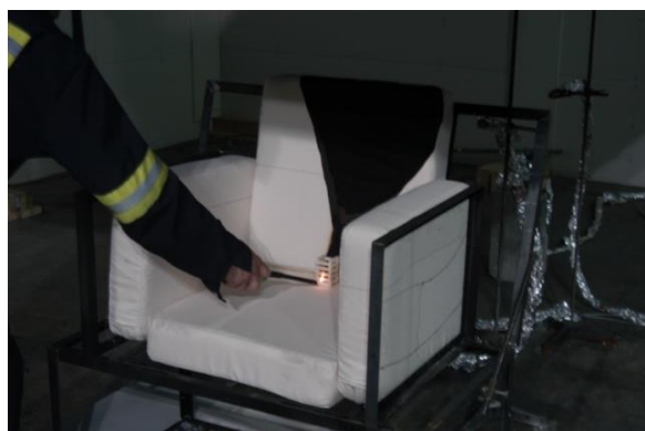
Figure 15. Two photographs show an Ignition Source 5 wood crib on a chair mock-up as it was ignited (left) and the resulting flame 57 s later.
