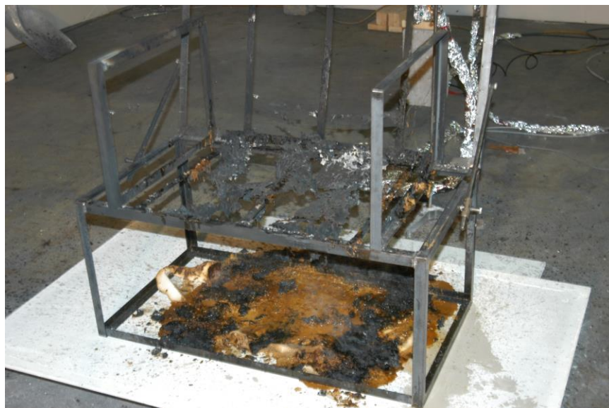
Figure 74. Photograph showing the residue on the test stand and support base following Test 14_2.
