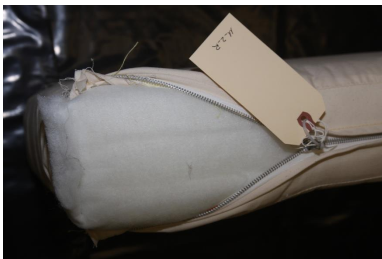
Figure 6. Photograph showing the corner of an FPUF slab wrapped in PEFW and placed inside a cotton outer cover.
