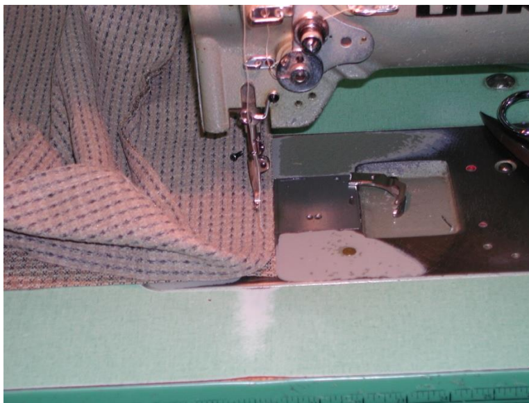
Figure 4. Photograph showing the bottom and sidewalls for a cushion cover being sewn together. The top seam has already been completed.
