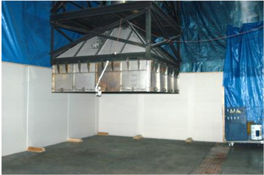
Figure 1. Photograph showing the collection hood for the 1 MW FPC used during the experiments.
