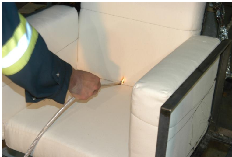
Figure 13. Photograph showing ignition of a furniture mock-up with Ignition Source 1.
