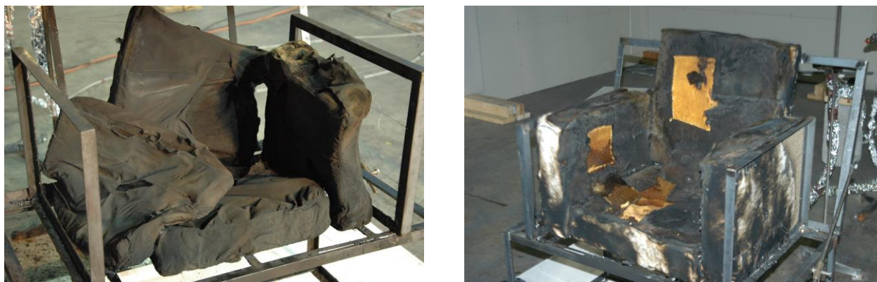
Figure 115. Two images showing the remaining charred material on the mock-up stand following Test 5_3 (left) and Test 6_1 (right). Sections of the cover and barrier fabrics have been cut out to expose the material underneath in the figure on the right.
