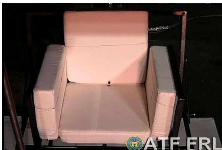
Figure 24. This frame taken from the Video Camera #3 view of the mock-up during Test 9_2 shows the appearance of the cotton fabric immediately following the removal of Ignition Source 1.
