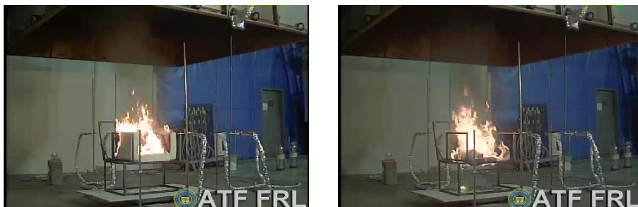
Figure 32. Two frames taken from a video recorded by Camera #8 show the appearance of the fire during Test 13_2 at 723 s (left) and 855 s (right) following application of Ignition Source 1.
