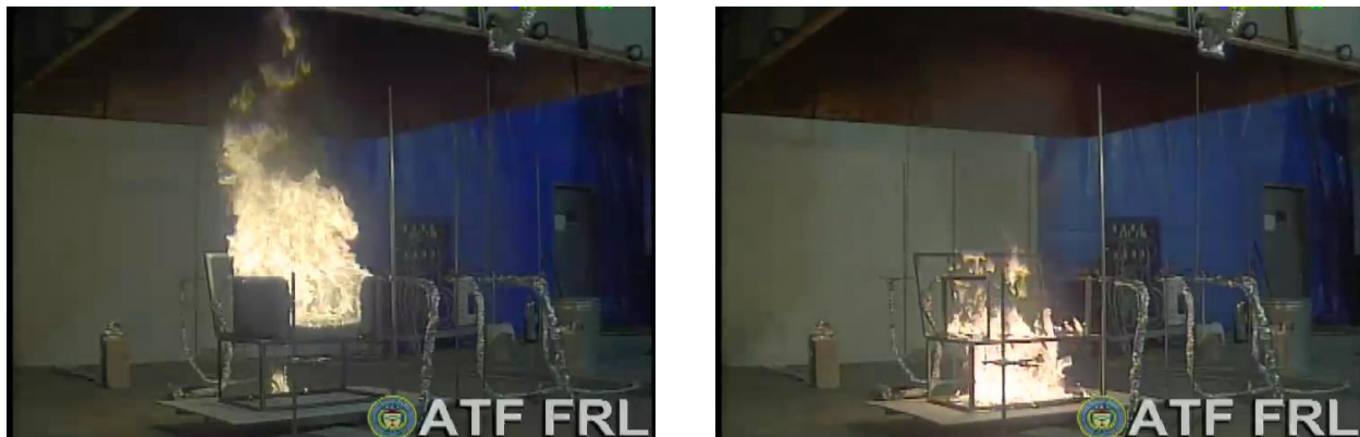
Figure 29. Two frames taken from a video recorded by Camera #8 show the appearance of the fire during Test 10_1 at 146 s (left) and 220 s (right) following application of Ignition Source 1.
