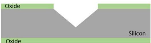
2) Silicon KOH etching to form V-groove
