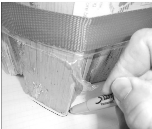
Figure 8. Tracing the Perimeter of the Wood.
