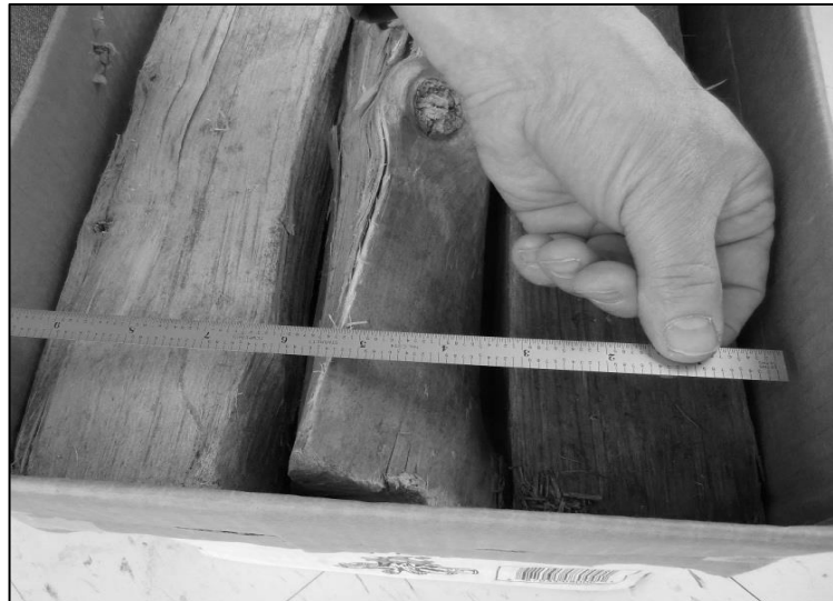
Figure 3.a. – Measuring the Width of the Firewood in a Box
