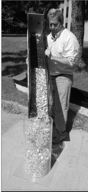
Exhibit 6. Filling a 44 L Test Measure.
