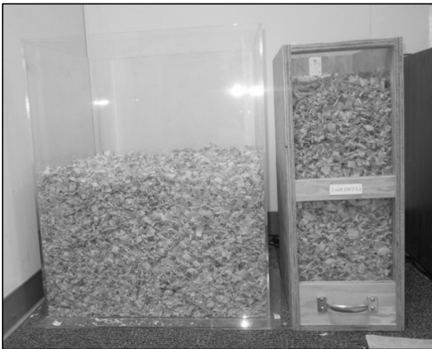
Exhibit 20. Test Measures Used in Study. The large test measures hold up to 279 L (10 cu ft) while the small measures hold up to 52 L (1.5 cu ft).
