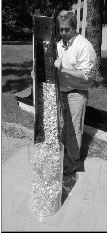
Exhibit 6. Filling a 44 L Test Measure.
