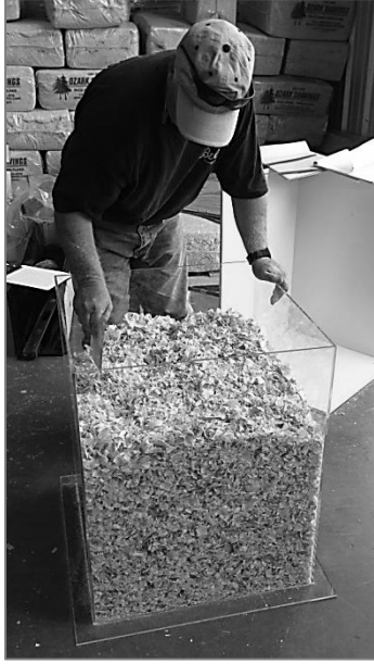
Exhibit 28. Leveling the Surface. Showing the use of a 150 mm mesh to level the surface of large flake bedding.
