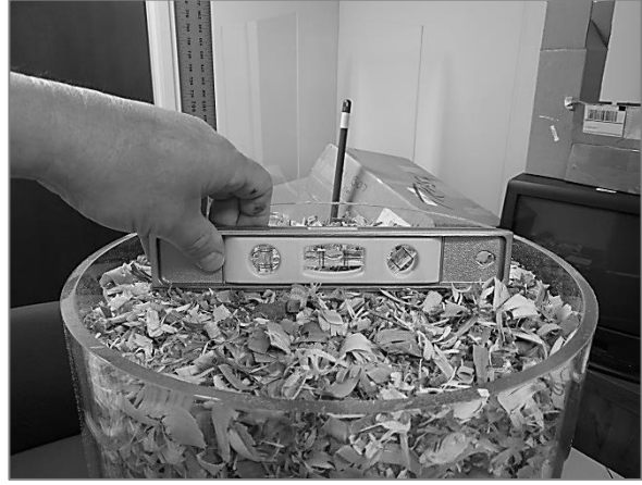
Exhibit 29. Checking Level. Checking the surface of large flake bedding for an approximation of a level condition.
