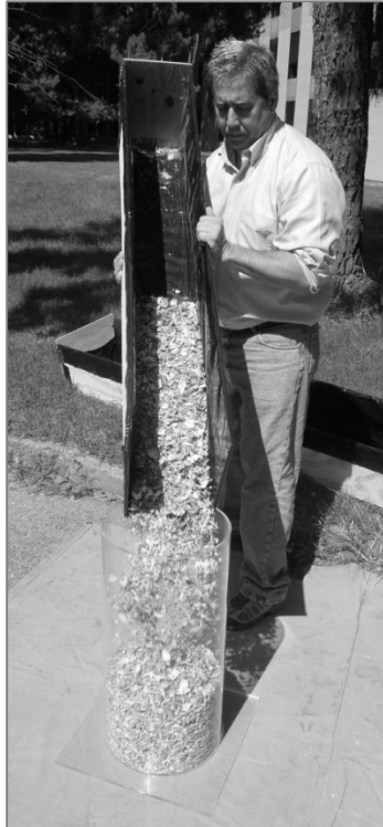
Exhibit 15. Filling a 44 L Test Measure.
